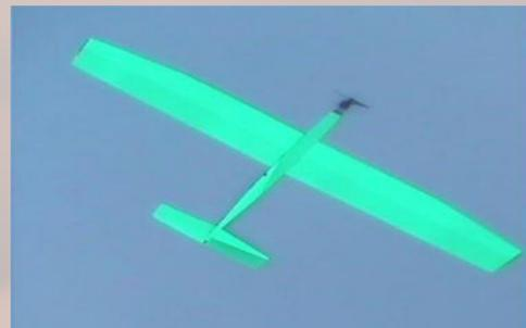
This project studies using LED light strips wired in series to reduce the required power supply and decrease the weight penalty of the system.
