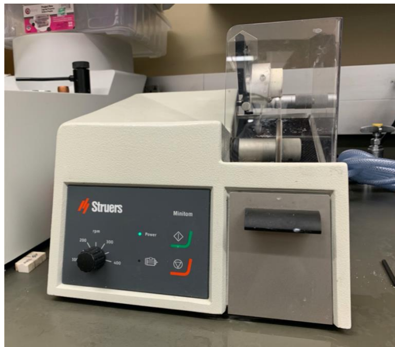
Figure 4.3 Struers Minitom slow-action diamond saw was used to cut thin membranes from cylindrical cast samples.
