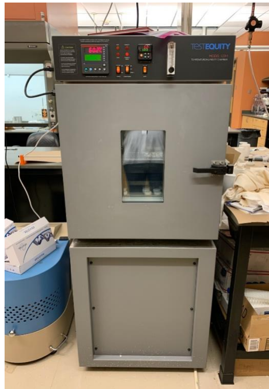
Figure 3.11 Temperature and humidity control chamber used for geopolymer composite processing.
