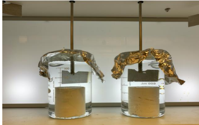
Figure 5.2 Experimental set up for leaching tests on geopolymer sample with encapsulated solid waste from produced water inside (left) and the control pure geopolymer sample (right).
