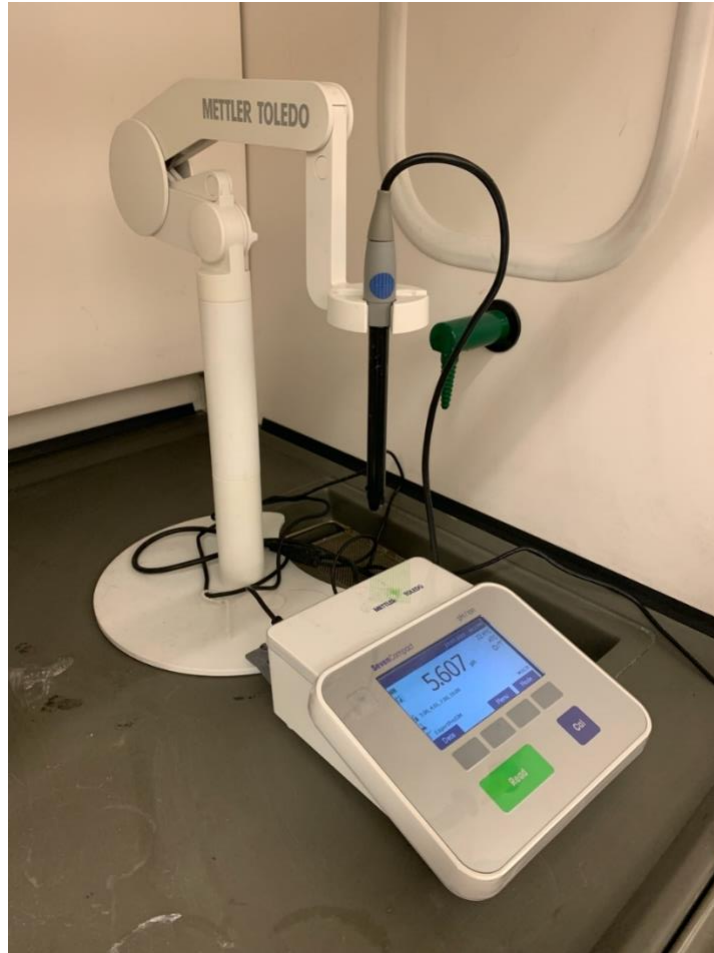
Figure 3.13 SevenCompact pH meter S220 was used for pH measurement of water samples.
