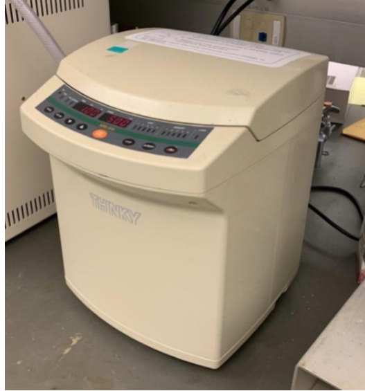
Figure 3.10 ARE-310 Thinky mixer used for geopolymer composite processing in this research.
