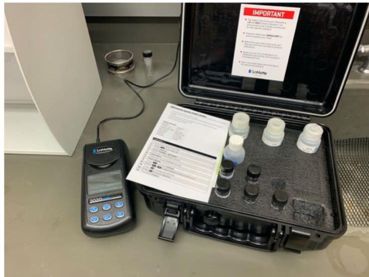
Figure 3.15 The LaMotte 1970-EPA Model 2020we Portable Turbidity Meter (LaMotte Company, Chestertown, MD).
