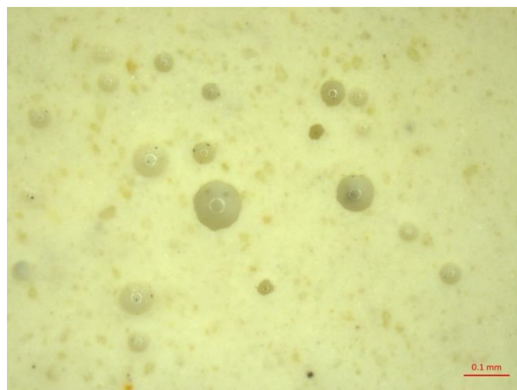
Figure 4.11 Optical micrograph of the geopolymer+zeolite composite membrane with 10 vol % fine zeolite.
