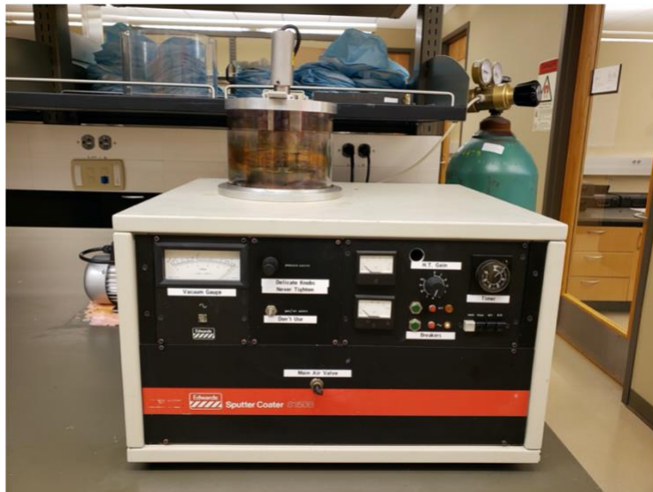
Figure 3.18 The Edwards Sputter Coater S150B (Edwards Vacuum LLC, Albany, NY) that was used for this study to coat Au on powder/granular and solid membrane samples. .
