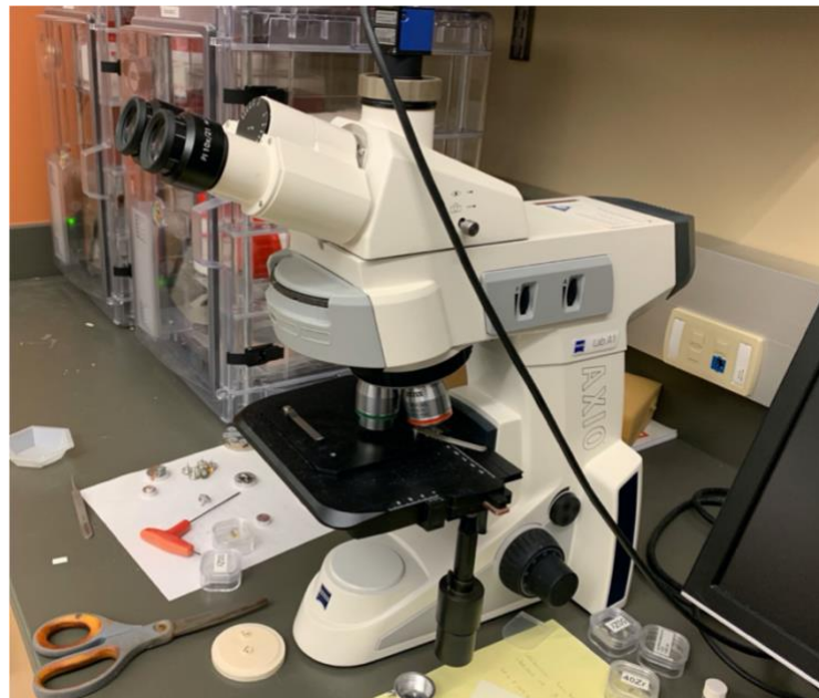
Figure 3.16 The Carl Zeiss' AxioLab A1 Modular, upright Optical Microscope for Materials Science (Carl Zeiss Microscopy, LLC, White Plains, NY) that was used for this study. .
