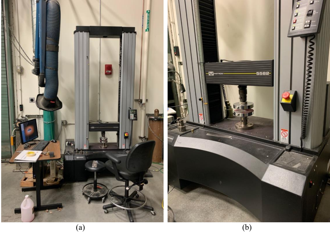
Figure 3.23 (a) Photograph of the Instron Universal Testing System, and (b) Load cell and sample mounting fixtures, used for measuring the compressive strength properties of the geopolymer and geopolymer composites in this study.
