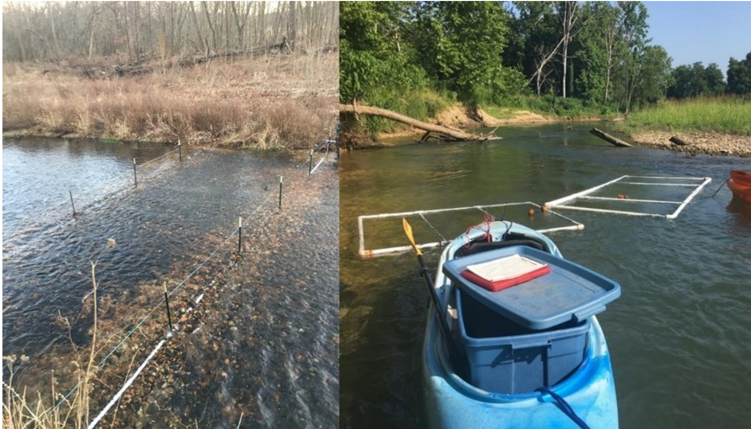
Figure 2. Fixed array constructed at upper end of study segment (left) and floating array used for active tracking (right) in Spavinaw Creek. At fixed array sites, two antennas were placed parallel to one another to determine directional movement of each fish passing through the antenna. The floating array consisted of two antennas housed in floating PVC towed behind kayakers. Both fixed and floating arrays were connected to a multi-antenna reader (Oregon RFID; Portland, Oregon) and powered using a 12-volt deep-cycle battery.
