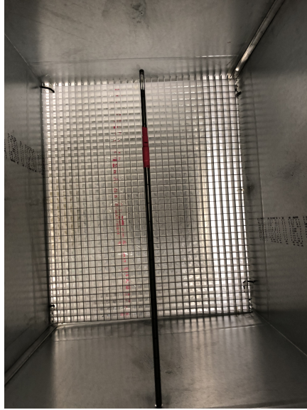
Figure A.7: Duct with air straightener
