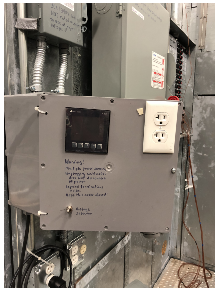
Figure A.2: Aplus meter for power measurement
