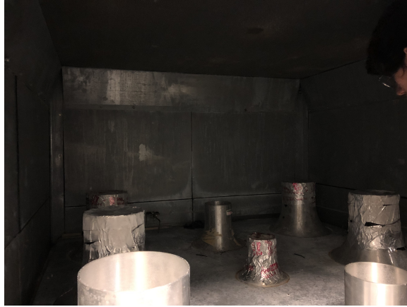
Figure A.14: Indoor psychrometric chamber nozzle sets
