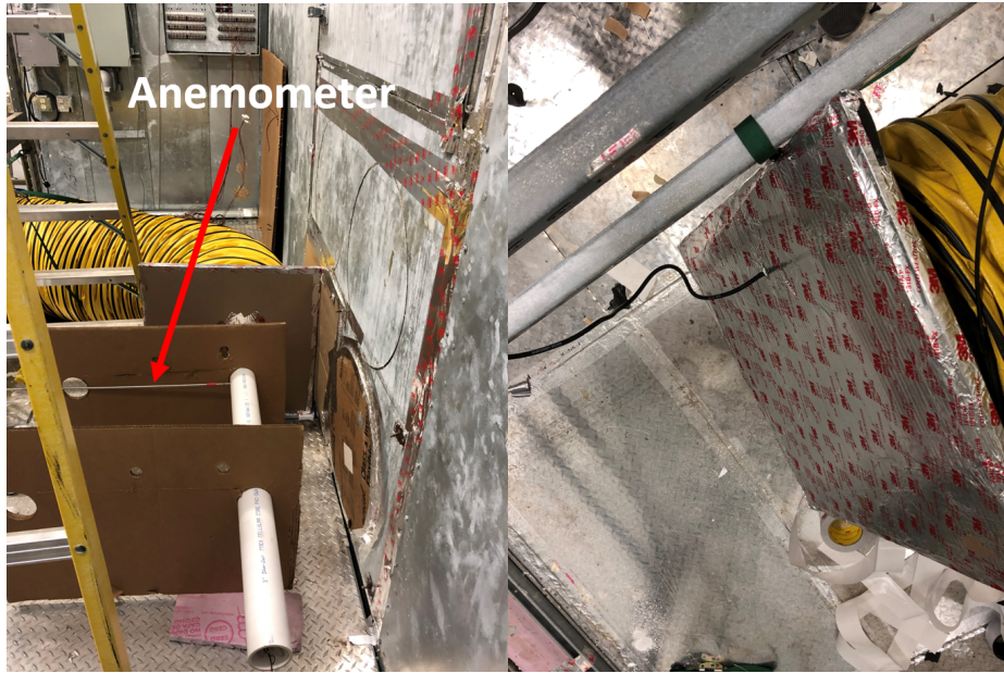
Figure 5.2: Leak testing setup
