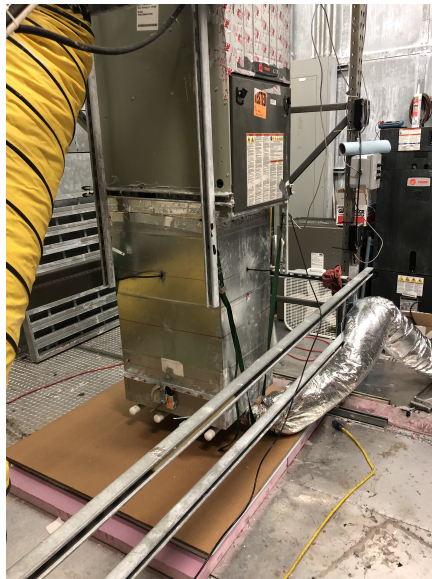
Figure A.22: Reduced floor distance with cardboard (standard duct case)
