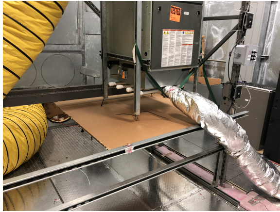
Figure A.11: Reduced floor distance with cardboard (no duct case)
