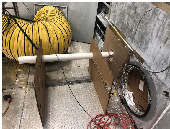
Figure A.16: Test setup for leak testing (code tester side)
