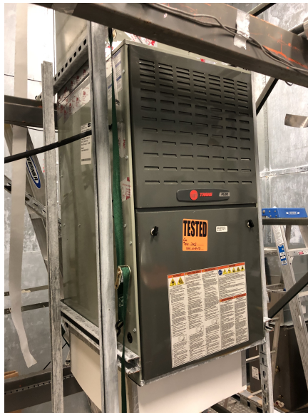
Figure A.18: Furnace section of test unit
