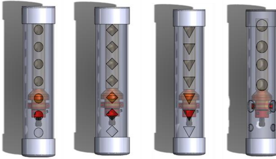
Figure 74: Test matrix of inlet shape and location used for K45 sizing on prototype
