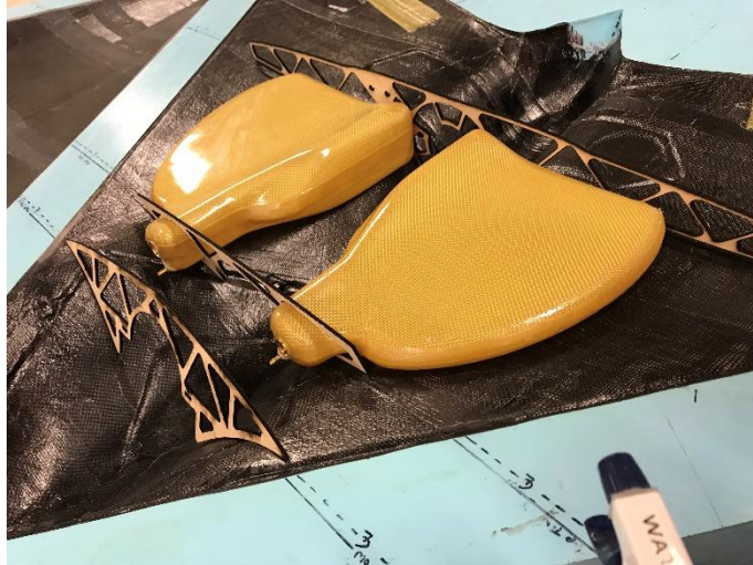
Figure 36: Test fitting the fuel tanks with the primary structure on a prototype airframe.
