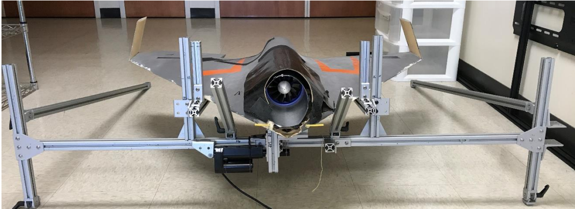
Figure 58: Beast on launcher for fine-tuned placement of all support structure
