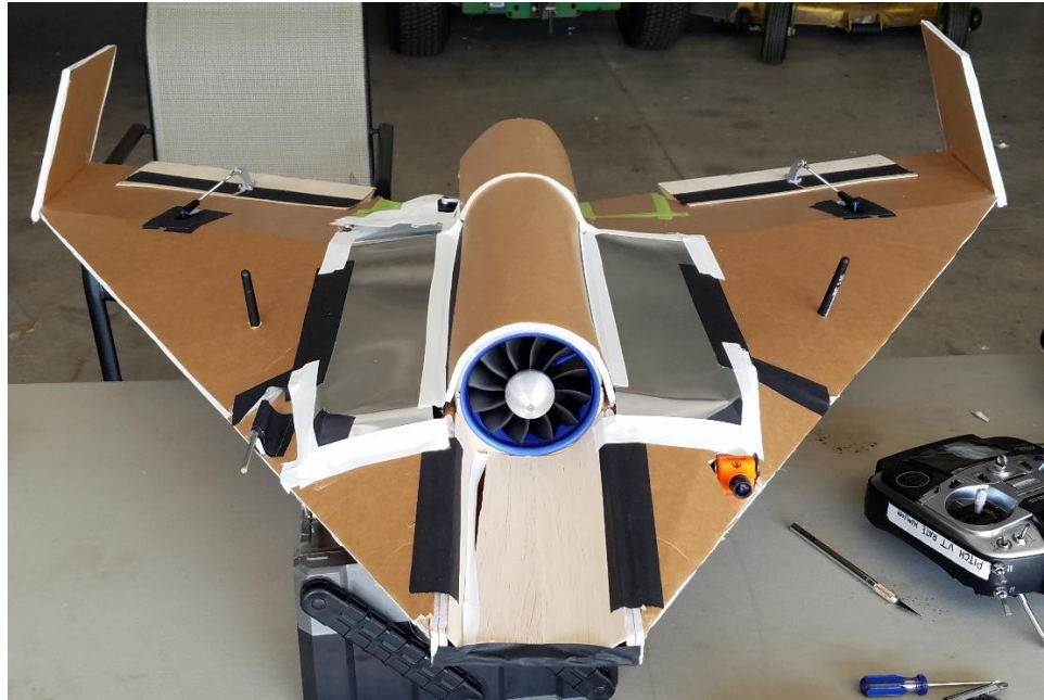
Figure 95: Final foamboard model that simulates full composite airframe
