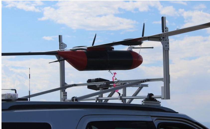
Figure 22: Roof-Mounted Cable Release Example (University of Colorado Boulder)
