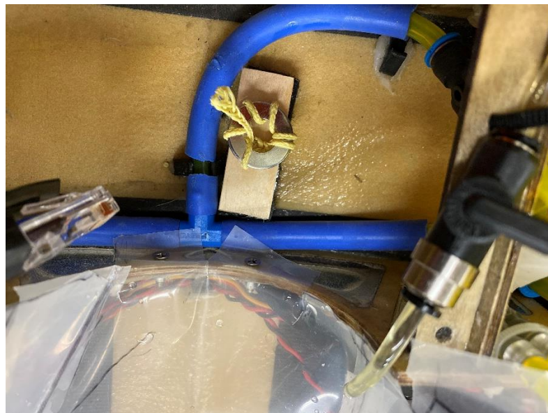
Figure 39: Shielded fuel tubing under turbine and secured to skin. Also visible is the launcher attachment line with nose Mylar screw locations.
