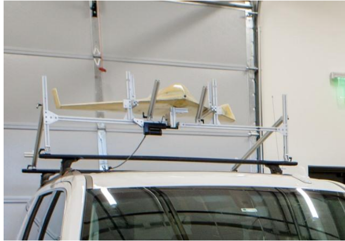
Figure 70: TIA mounted on launcher for sizing
