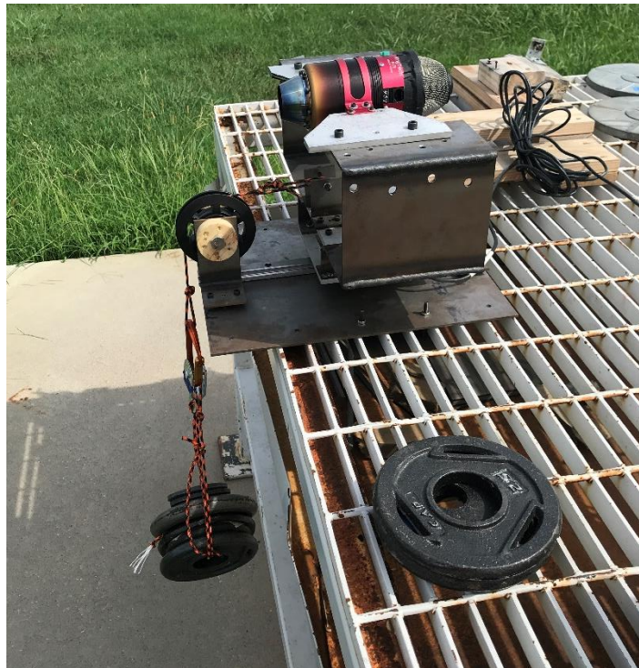
Figure 80: K70G2 turbine used on TIA mounted to thrust cell undergoing calibration
