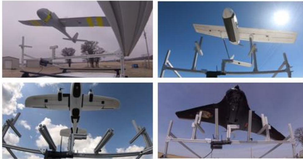
Figure 56: All four tested aircraft exhibiting roll on release except for the Believer (lower left)
