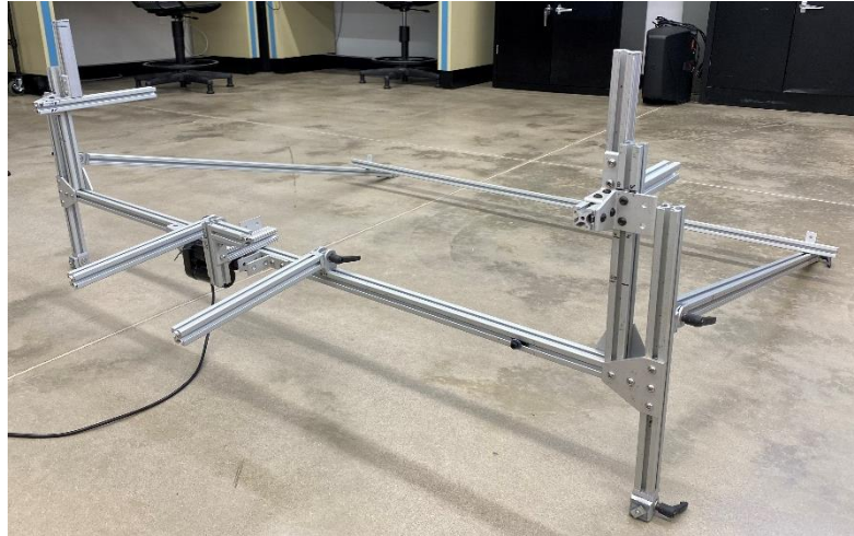
Figure 54: Launcher with delta wing modification installed
