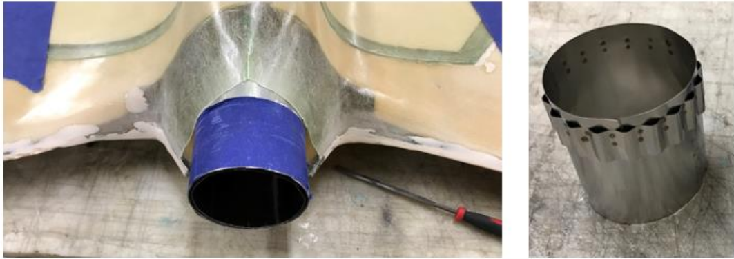
Figure 38: Sizing and trimming of the jet pipe
