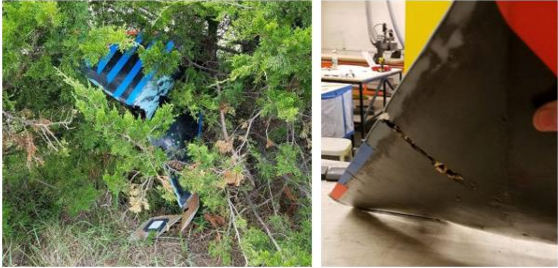
Figure 30: Damage to test aircraft from small trees and barbed wire fence at 70+ mph due to turbine failure
