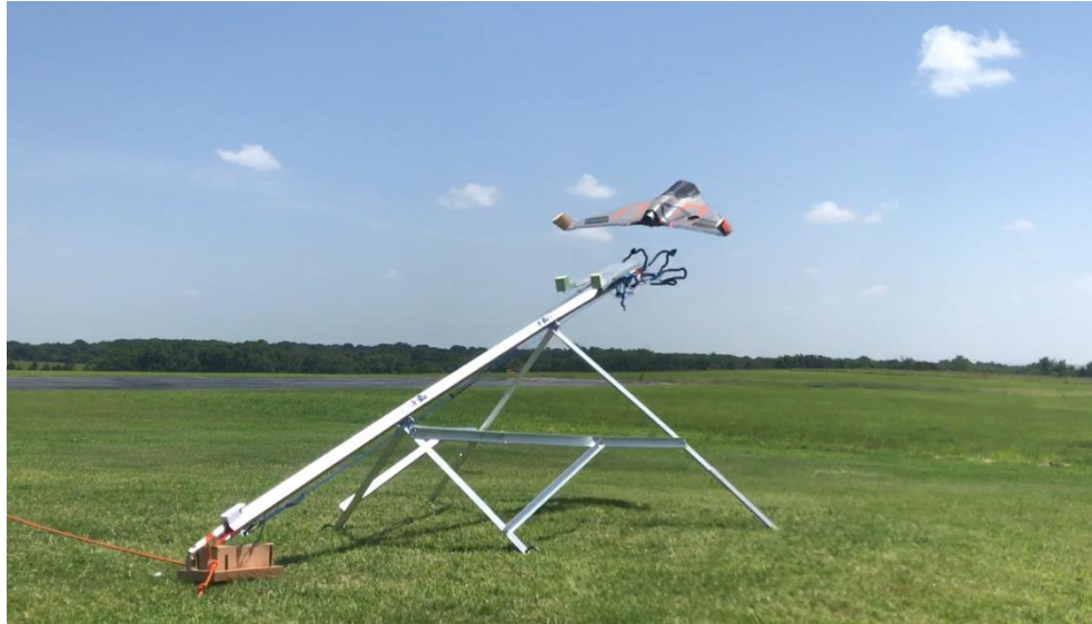
Figure 21: Catapult launch example (bungee propelled)
