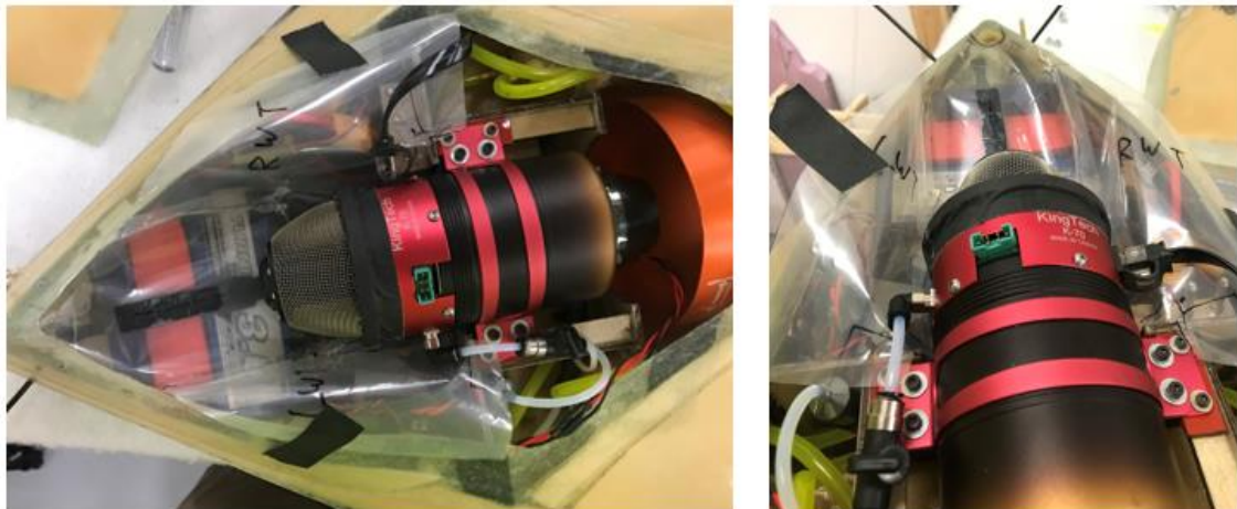
Figure 41: Mylar shielding in the nose of the airframe
