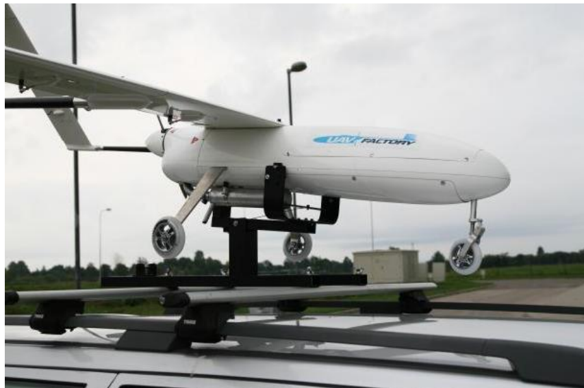
Figure 23: Pivoting Pin Release Example (UAV Factory) 35
