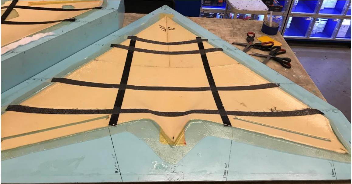
Figure 85: Bottom skin after layup but before removal
