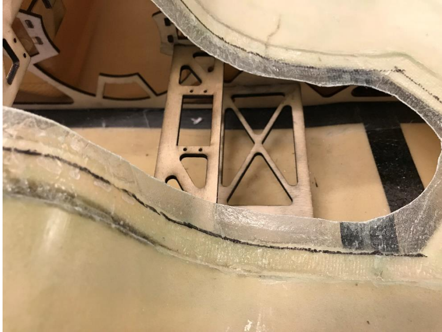
Figure 90: Rear starboard avionics bay prior to component installation.
