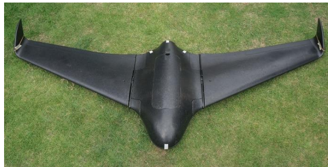
Figure 53: Skywalker X8, 2120 mm wingspan, pusher prop 45
