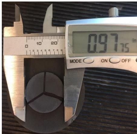
Figure 10 - Measuring the diameters to be averaged and used to calculate the tensile bond strength.
