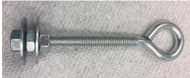
Figure E. 1 - Tensile bond strength load frame connection anchor.
