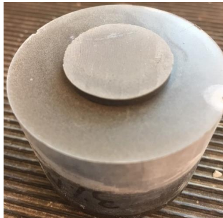
Figure 9 - Tensile bond strength post analysis of complete bond failure at the material interface.
