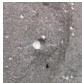
Figure B. 1 - Closed up image of pore in a nanoparticle barite sample.
