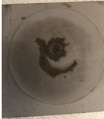
Figure 8 - Tensile bond strength post testing analysis revealing failure away from the material interface.
