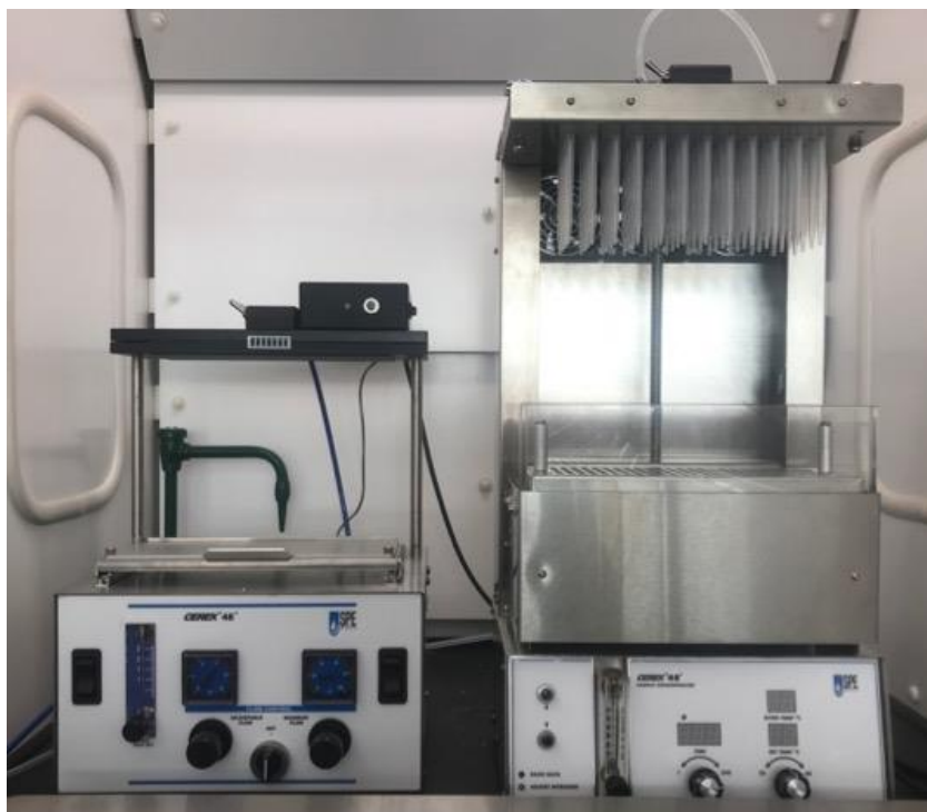
Figure 1. A picture of the SPEware Cerex 48 positive pressure manifold and sample concentrator used to perform SPE on the wastewater samples. On the left is the positive pressure manifold used to applying nitrogen gas for loading samples and drying the SPE cartridge sorbent. On the right is the sample concentrator used to accelerate the evaporation of the elution mixture.
