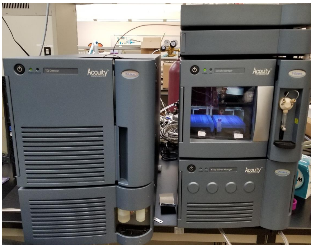
Figure 2. A picture of the Waters Acuity Classic UPLC-MS/MS system used to analyze the wastewater samples in this study. On the right are the UPLC pumps, autosampler, and column oven. On the left is the tandem quadrupole detector (TQD).
