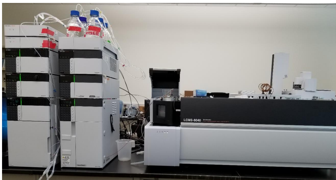
Figure 4. A picture of the Shimadzu 8040 UFLC-MS/MS system used to analyze the wastewater samples in this study. On the left are the UFLC pumps, autosampler, communications bus module, UV-VIS detector, and column oven. On the right is the tandem mass spectrometer.
