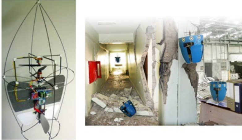
Figure 30: AirBurr and concept of operation [17].
