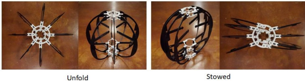
Figure 183: Foldable frame prototype for compact ATLAS design.
