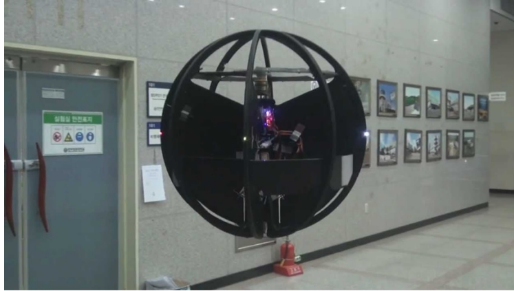
Figure 14: Korea's Spherical Flying Vehicle (SFV) - Singlecopter with four control Vanes [8].
