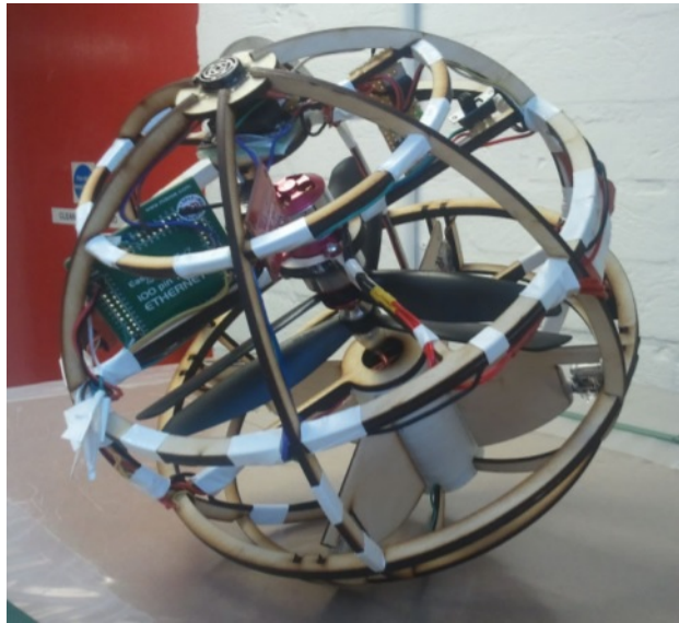
Figure 19: Contra rotating propeller with 4 control vanes [12].
