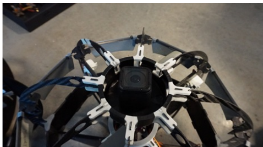
Figure 177: A GoPro session4 mounted on top of the ATLAS for ceiling inspection.
