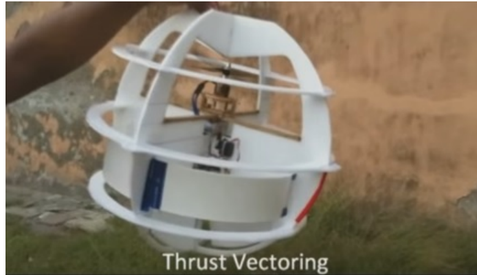
Figure 13: Hawk Eye - Single propeller with Thrust Vector and four control vanes [7].
