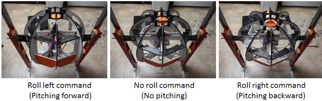
Figure 127: The vehicle is pitching forward or backward when roll left or right command input was introduced, respectively.
