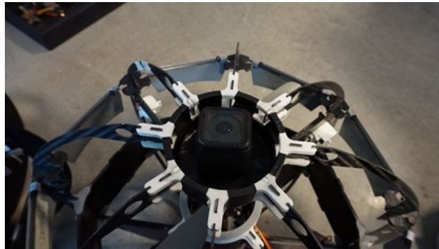
Figure 66: A GoPro Session 4 mounted on top of the top collar for indoor rooftop inspection.
