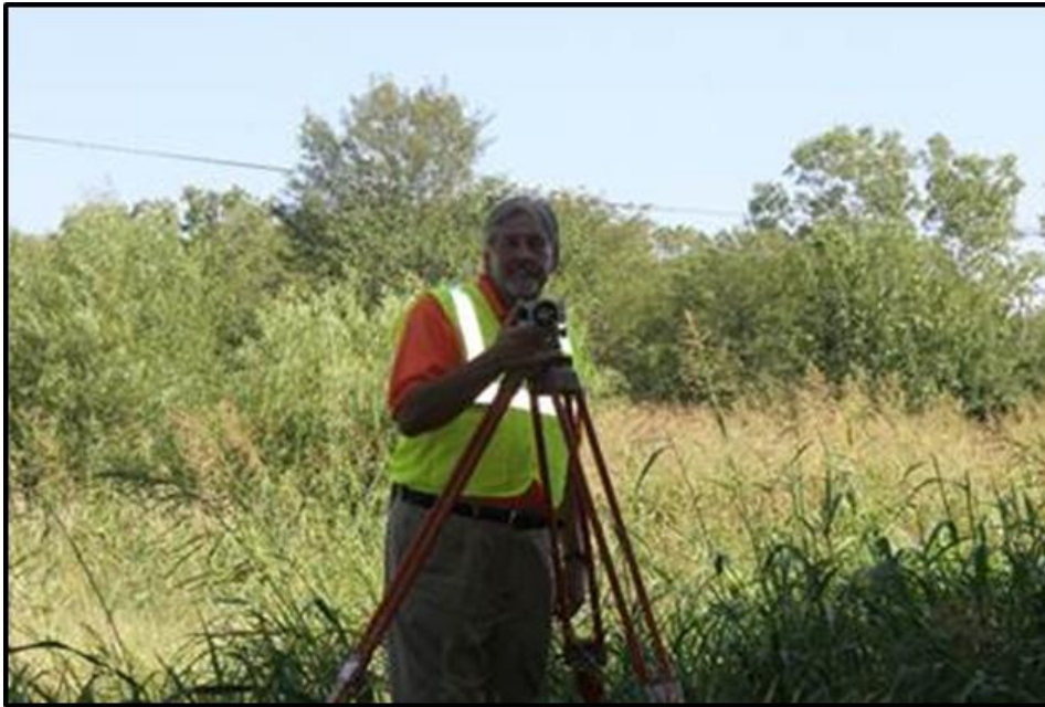
Figure 28. Elevations measurements made with traditional surveying equipment including an engineering level and a leveling rod.
