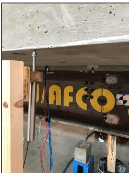
Figure 13. Installation of LVDT sensors on the laboratory prototype bridge
