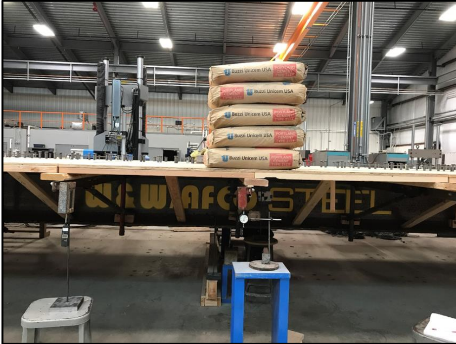
Figure 38. Cement Bag load testing performed on South Girder Walkway Platform
