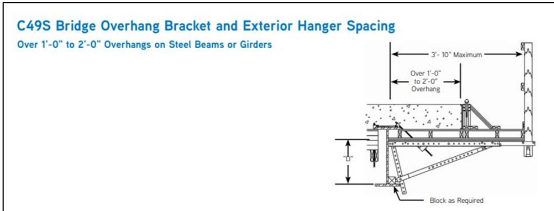
Figure 39. Typical C49S Bridge Overhang Bracket and Exterior Hanger Spacing (Dayton Superior Bridge deck Handbook)
