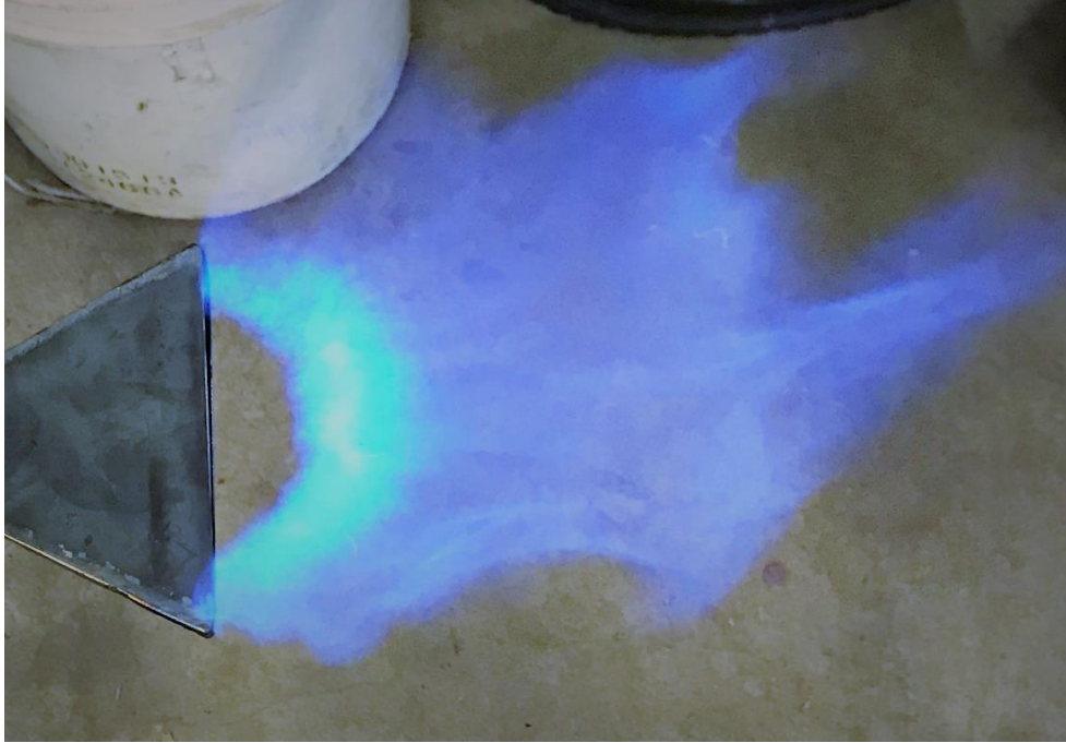
Figure 29. The blue flame generated by the burners
