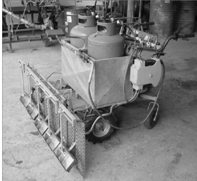
Figure 10. Self-propelled flaming machine (M. Raffaelli et al., 2013)
