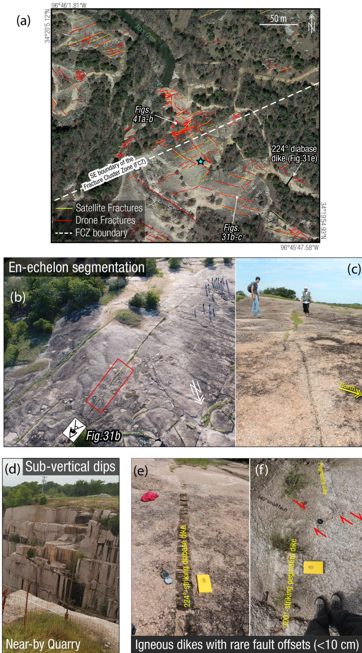
Figure 31. General characteristics of the fractures within the area. (a) Google Earth© satellite image of the study area, showing the satellite-scale (interpreted from the satellite image) and drone-scale fracture segments (interpreted from the drone images in Figures 28b-e). (b) Drone and (c) outcrop photographs of en echelon fracture patterns commonly observed in the study area. (c) Photograph of excavation at a nearby quarry (Martin Marietta Quarry) showing the sub-vertical geometries of the fracture systems in the exposed granitic basement rocks. (d) Photographs of fracture-filled igneous dikes and the observed small-offset faulting of some of the dikes.
