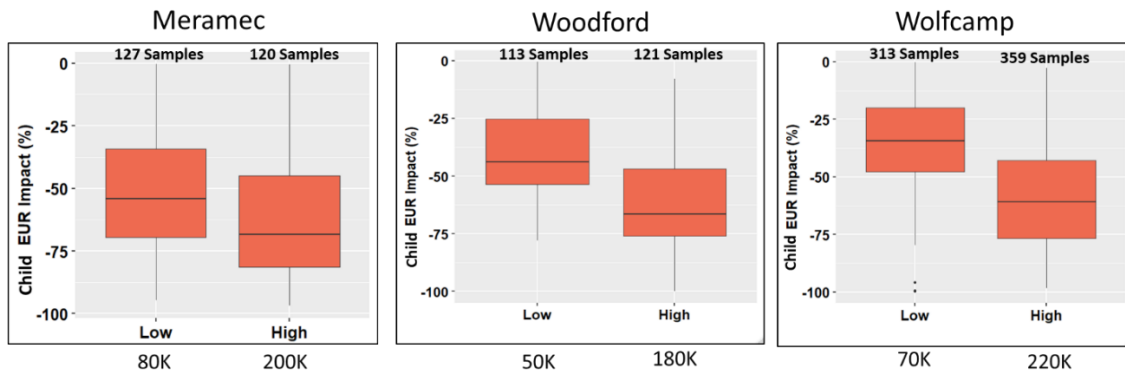
Figure 29: Impact of depletion on the EUR of child wells was studied using cumulative production by a parent well prior to frac hit as a proxy for depletion. The groups on the x-axis represent the parent well production before child well was drilled. The low group represents the average cumulative production of 50,000 to 80,000 bbl by parent well before child well is drilled. The high group represents the average cumulative oil production of 180,000 to 220,000 bbl. The figure shows that higher cumulative production by parent well (~ higher depletion) leads to higher negative impact on child EUR.
