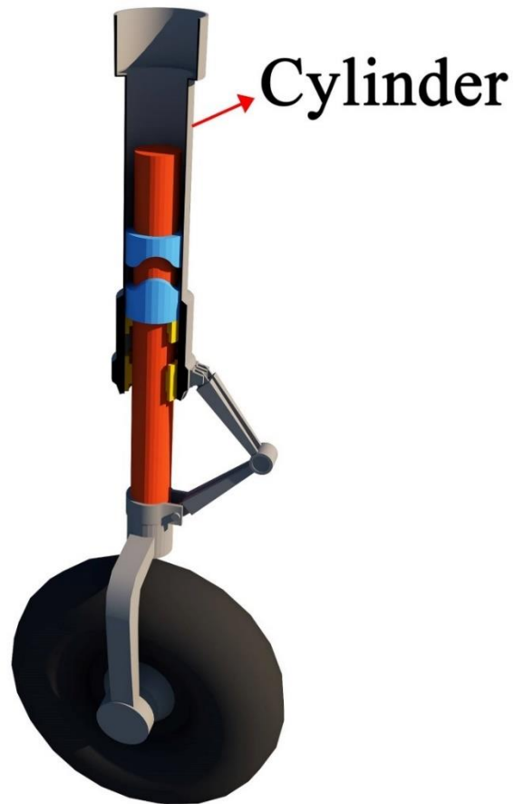
Figure 3.8. A model of aircraft landing gear with point out of a landing gear's cylinder.
