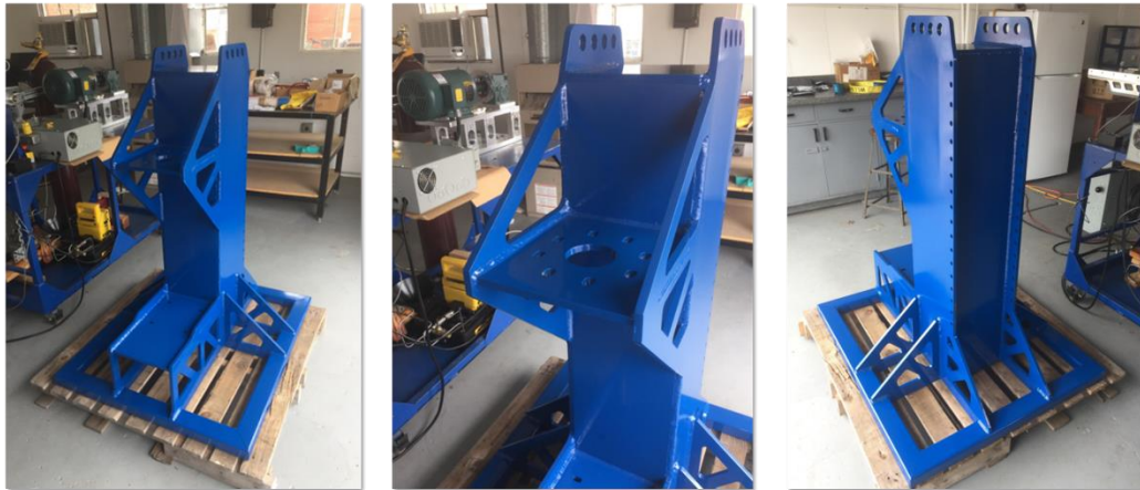
Figure 20: Steel frame of the testing setup
