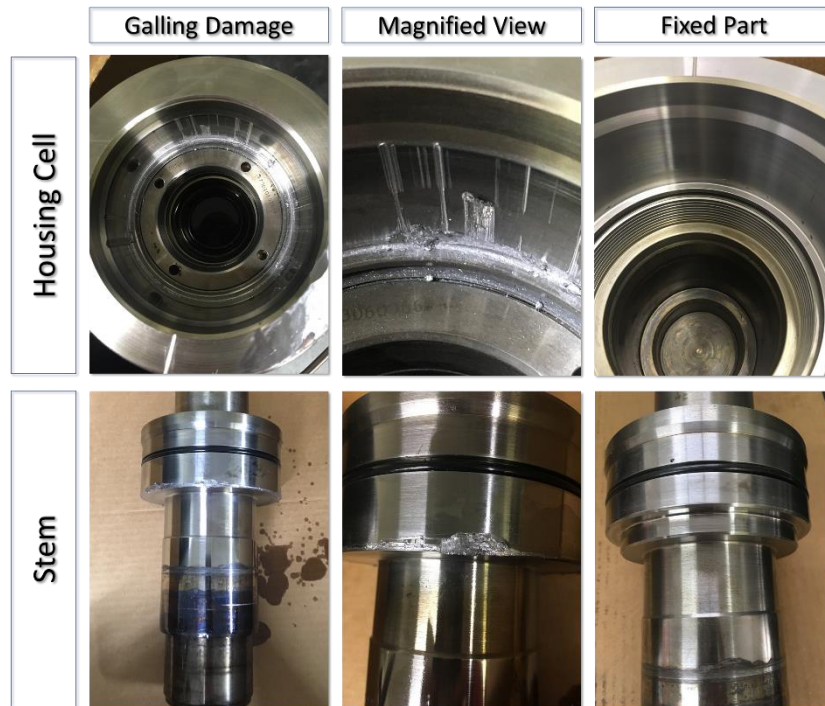
Figure 14: Stem and housing cell after galling
