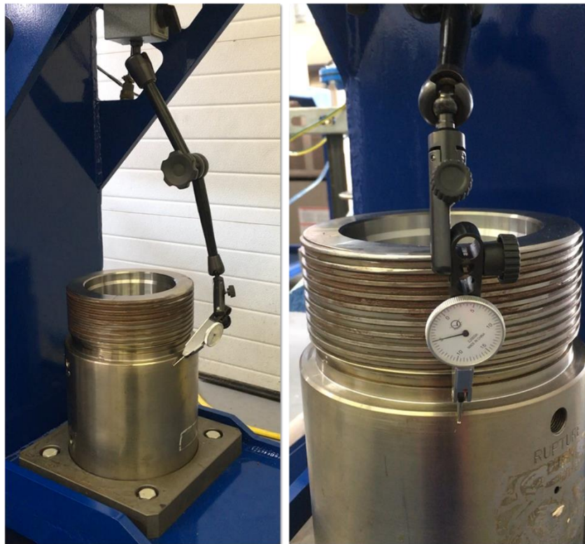
Figure 34: Housing cell alignment process
