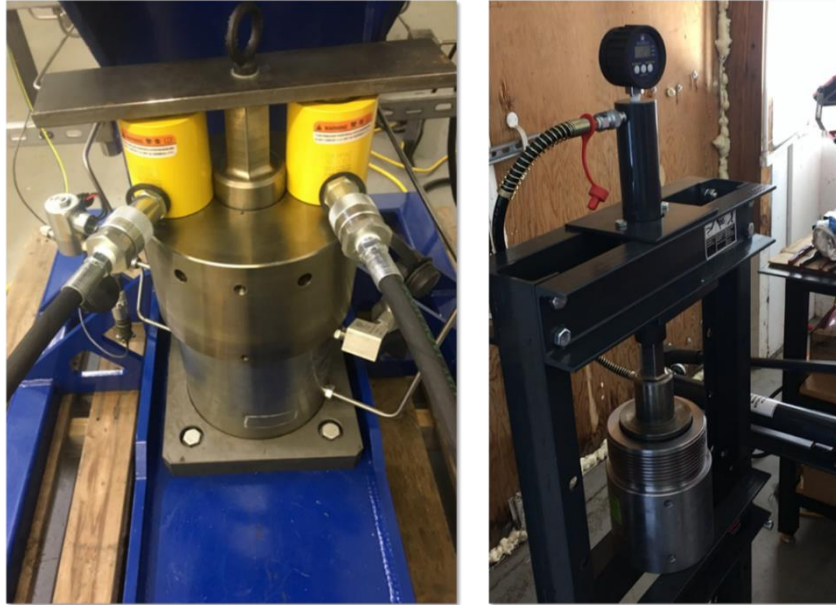
Figure 32: Metal seal installation and removal processes
