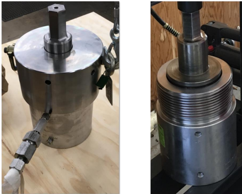
Figure 13: Fully assembled housing cell on the left and without a cap on the right
