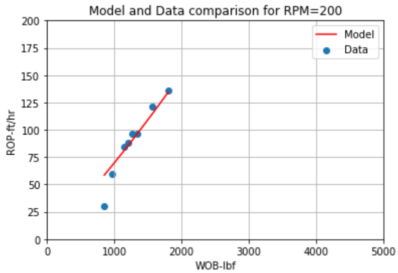
Figure 4.35. Comparison between the model and data ROP for four-bladed PDC bit at RPM=200 in BSS
