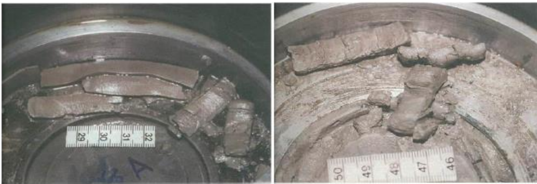
Figure.2.3. Shale ribbons for tests with water at 9000 psi CP and 0.011-inch depth of cut for polished (left) and non-polished cutter (right)(Smith, 1998)
