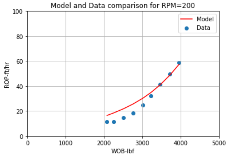
Figure 4.30. Comparison between the model and data ROP for five-bladed PDC bit at RPM=200 in SWG
