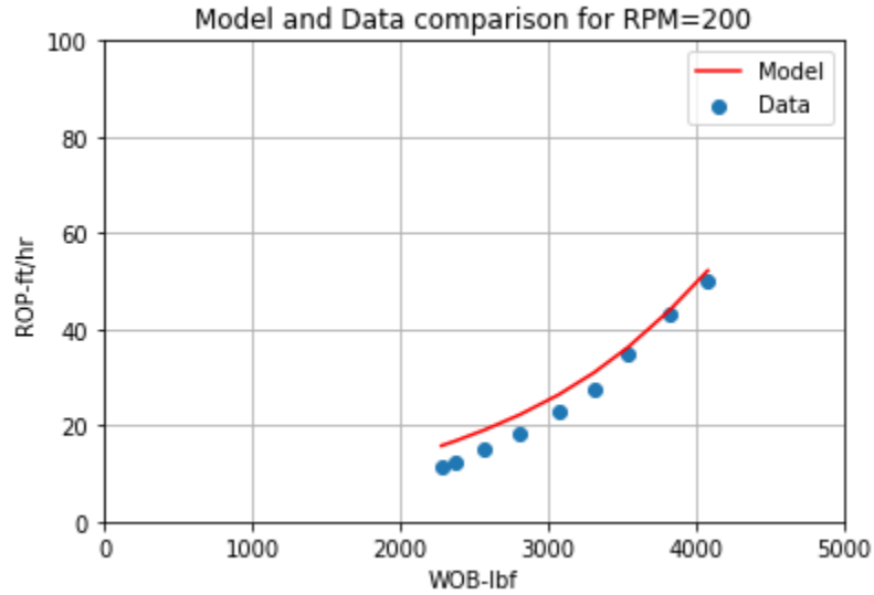
Figure 4.25. Comparison between the model and data ROP for four-bladed PDC bit at RPM=200 in SWG
