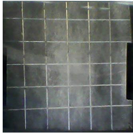
Figure 12. Testing the background signal of the dry membrane. This figure illustrates the background signal when membrane is dry.
