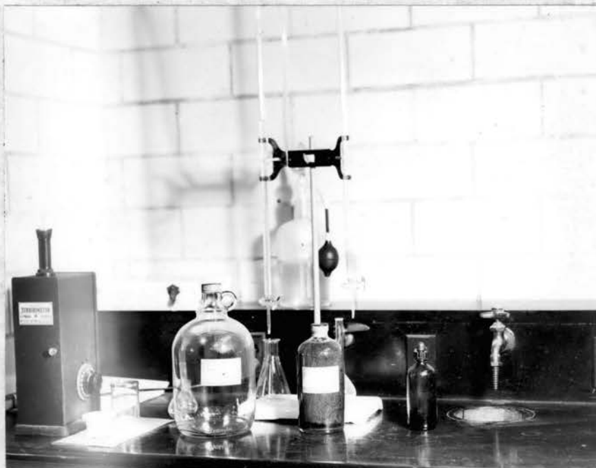
Fig. 8 - Standard titrating equipment used in determining hardness of water.
