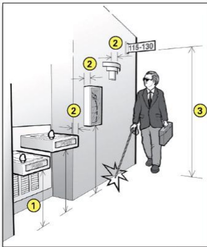
Overhead and wall-mounted objects that may be hazards along a pedestrian route
