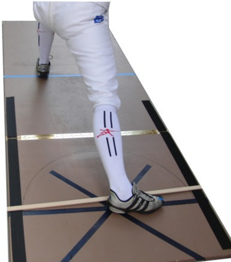
Figure 1. Testing platform for lunge testing. The bar acts as a kinesthetic reminder to maintain non-leading foot position.
