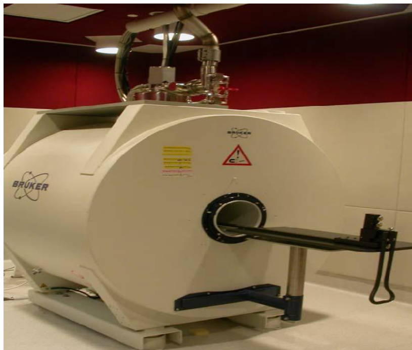
Figure 2.3. A 7.1 Tesla MRI system for small animal studies.
