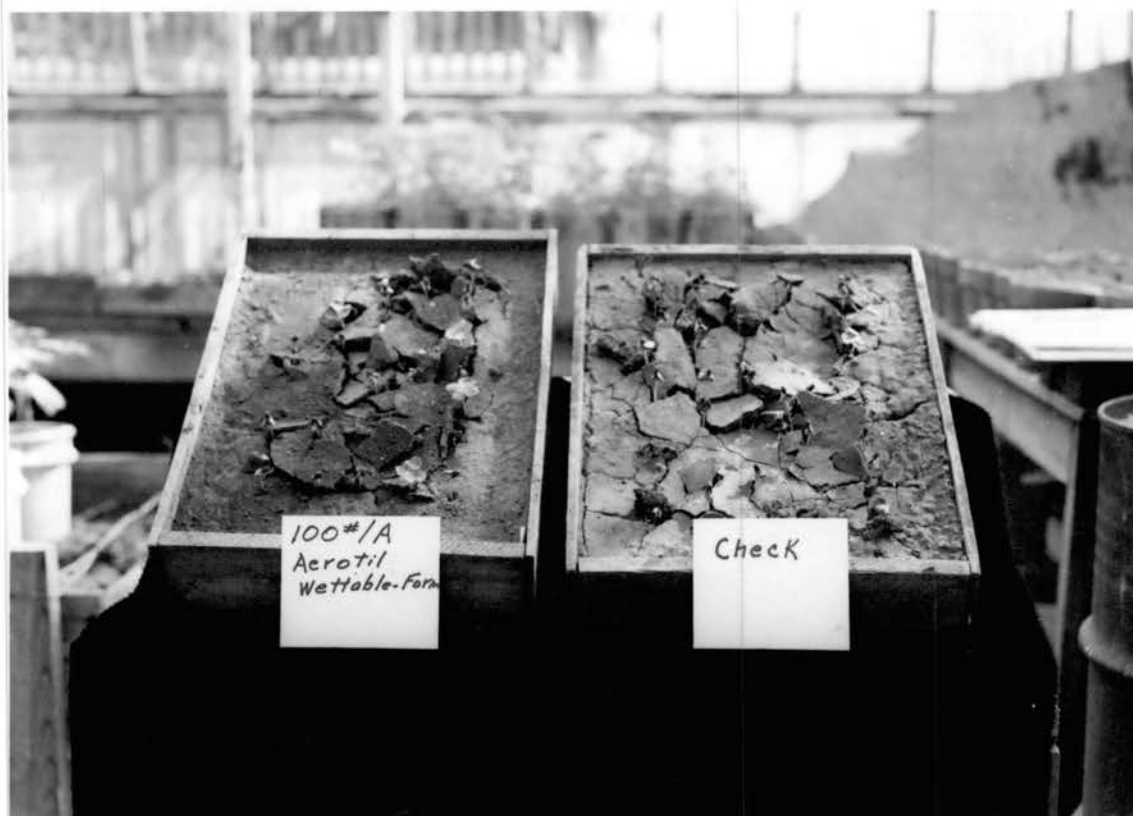
Fig. 3. Cotton emergence tests using soil treated with Aerotil wettable form (40 lbs./A. active ingredients).
