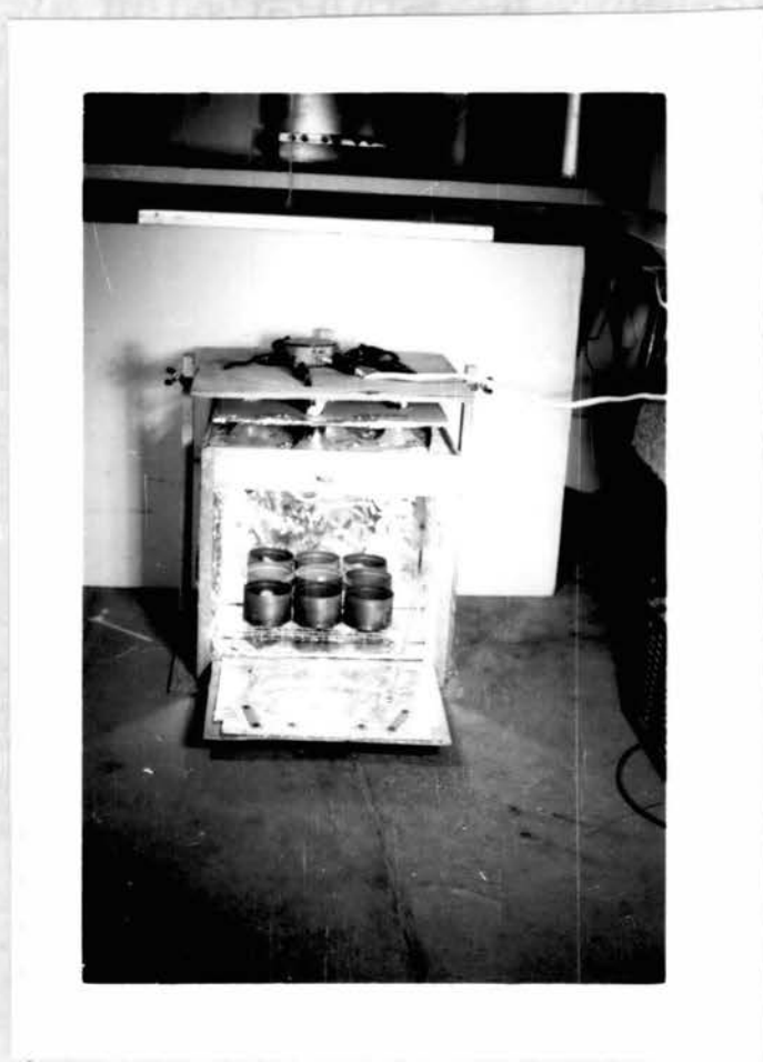
Figure 1--Experimental model infrared oven with nine standard 16 ounce soil sample cans
