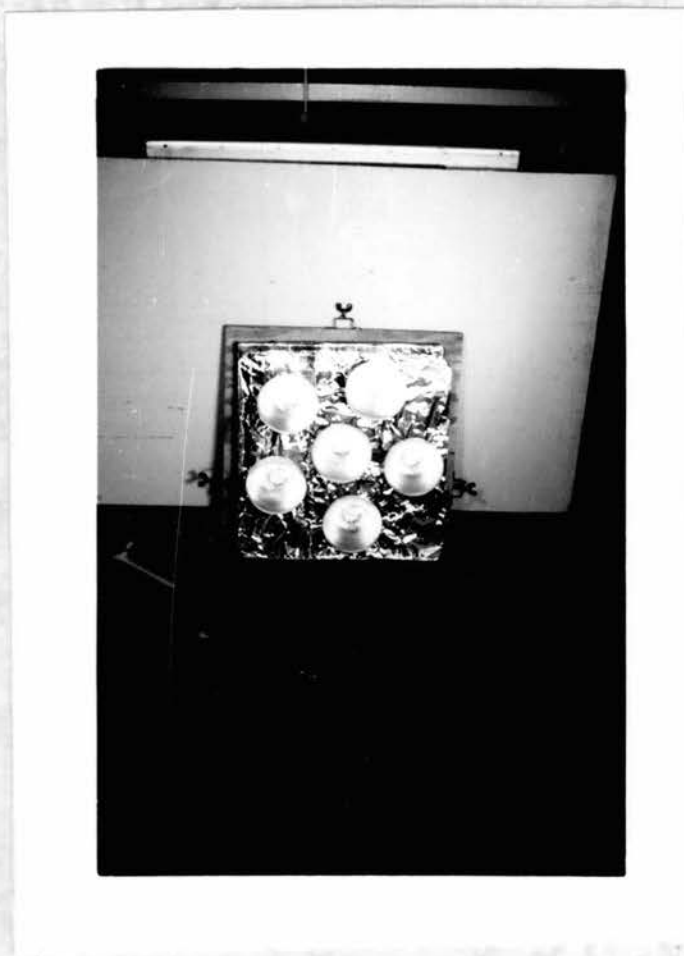
Figure 3--The oven top, underside showing the arrangement of the six lamps
