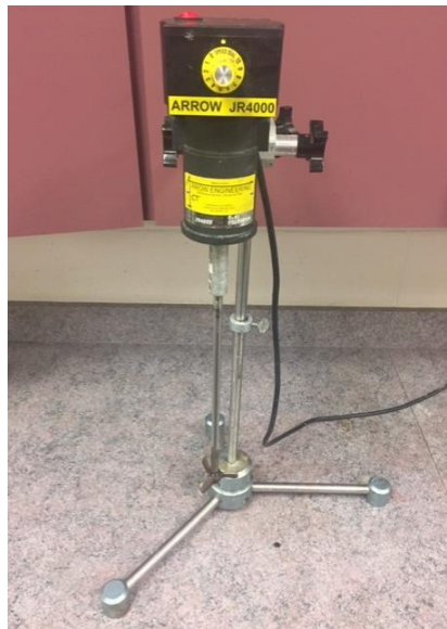
Figure 4.4: Variable speed benchtop mixer
