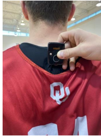
Figure 3. Inertial Measurement Unit (IMU) Placement.
