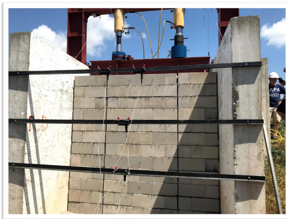
Figure 25 – Front of the test set up with the wire potentiometers Dismantlement
