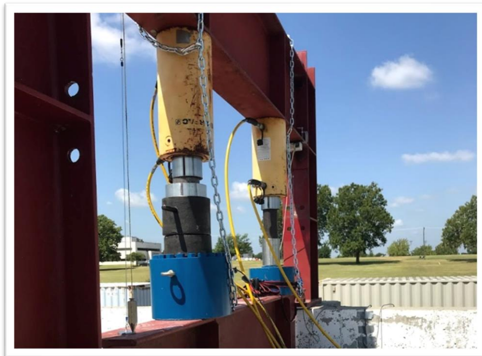
Figure 24 – Hydraulic cylinders, load cells and loading beam
