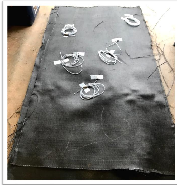
Figure 18 – Instrumented geotextile sheet before being put into a GRS model
