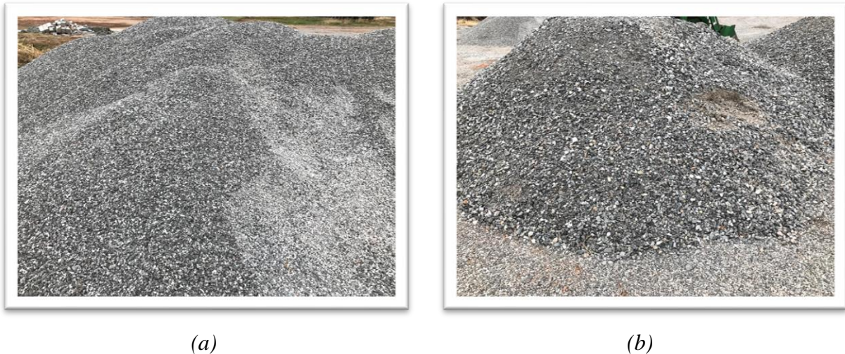
Figure 2 – Pile of aggregate at Fears Structural Laboratories: (a) 3/8" #2 Cover, (b) ODOT Type A
