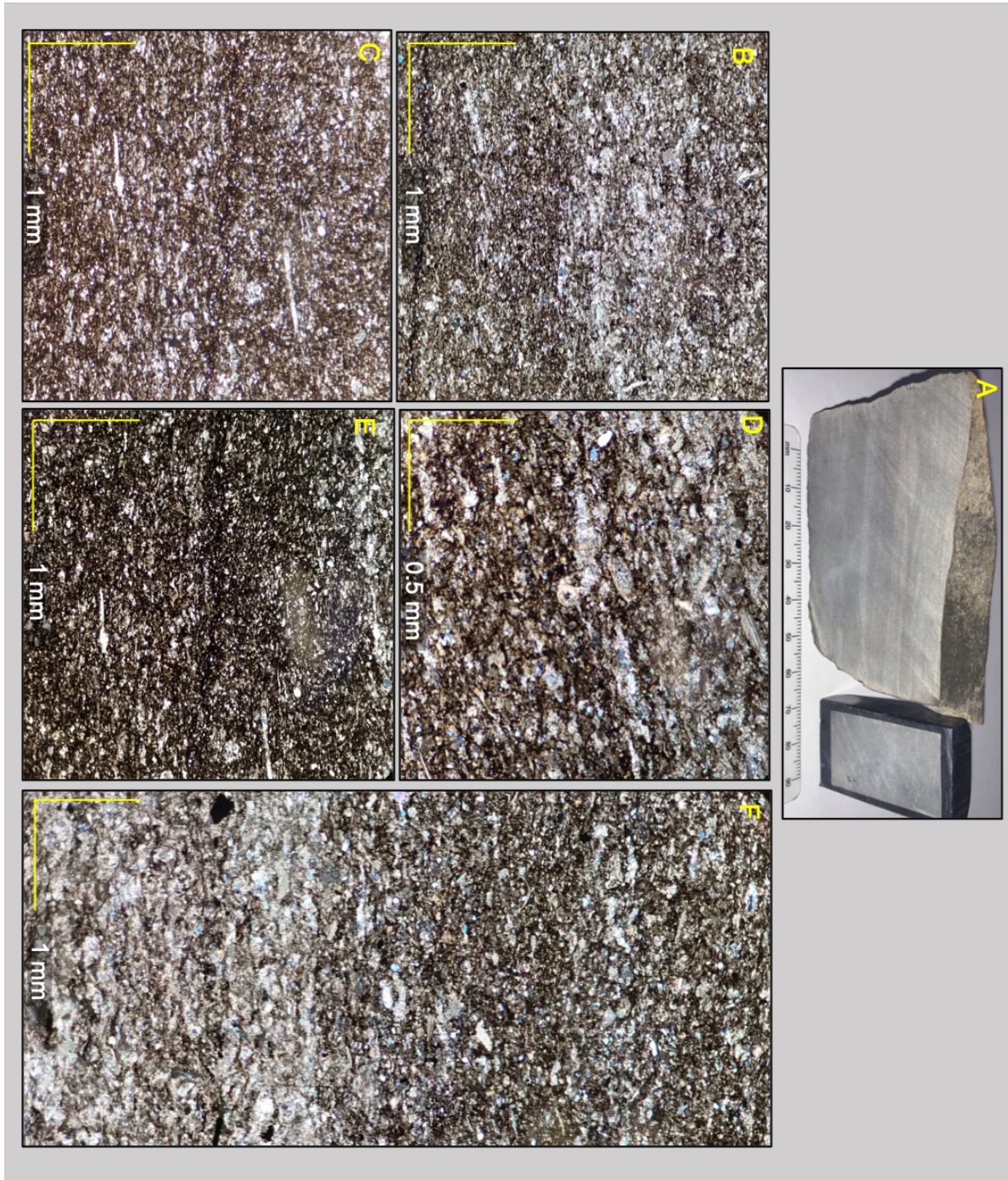
Figure 28. Petrographic analyses of sample taken at point 1D3. A) Hand sample. B) Thin section micro photograph taken in cross polarized light at 4X power. C) Thin section micro photograph taken in plane polarized light at 4X power. D) Thin section micro photograph taken in cross polarized light at 10X power. E) Thin section micro photograph C taken in cross polarized light at 4X power. F) Thin section micro photograph taken in cross polarized light at 4X power.
