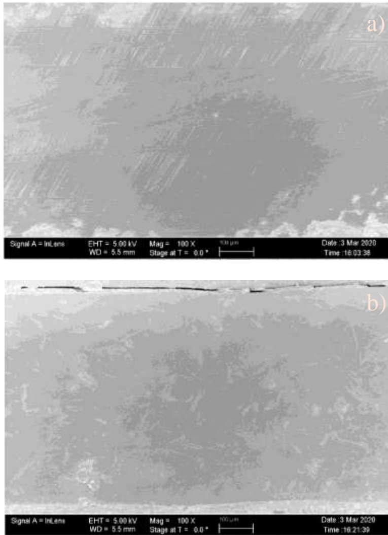
Figure 33: a) 15+5% graphite/ RIMR 135 + RIMH 137 at x100, b) 30+5% graphite/ RIMR 135 + RIMH 137 at x100
