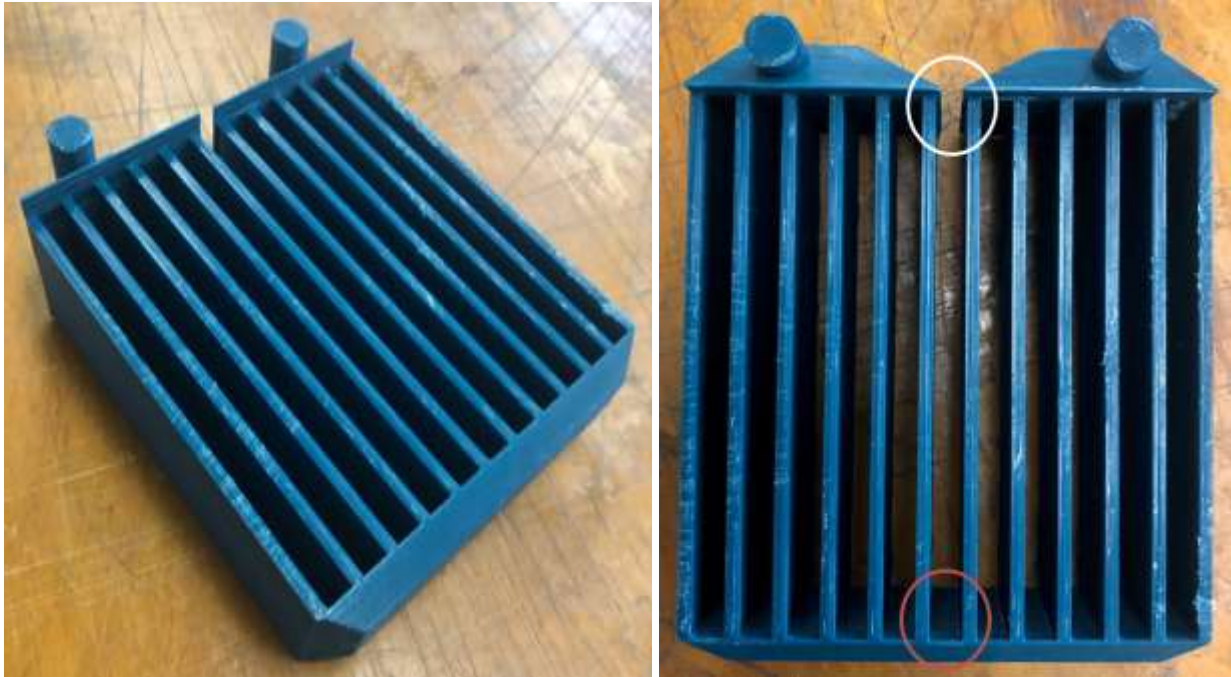
Figure 51: 3D printed flow channels. Part of the model that experiences the largest stress due to the top opening is circled in red.
