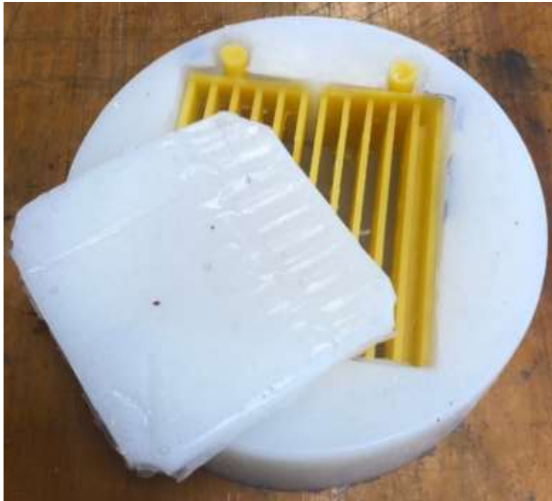
Figure 57: Silicone mold for heat exchanger fabrication, with wax flow channels that correctly fit the mold
