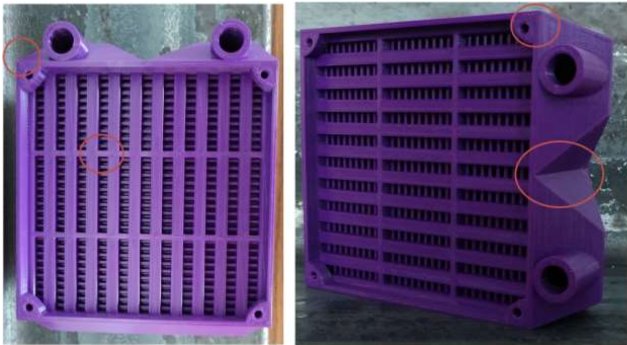
Figure 50: 3D printed heat exchanger model. Some parts of the model that have 90° corners and edges are circled in red
