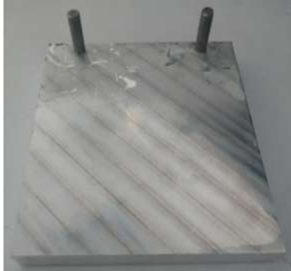
Figure 59: Aluminum fixture used to support flow channels mold
