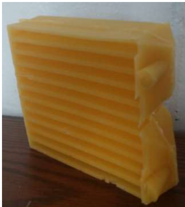
Figure 56: Solidified wax flow channels
