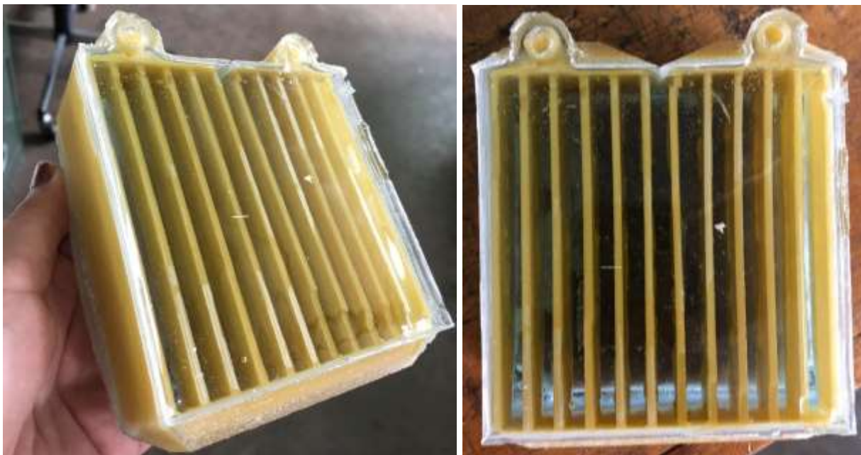
Figure 62: Compact neat epoxy heat exchanger prior to flow channels removal
