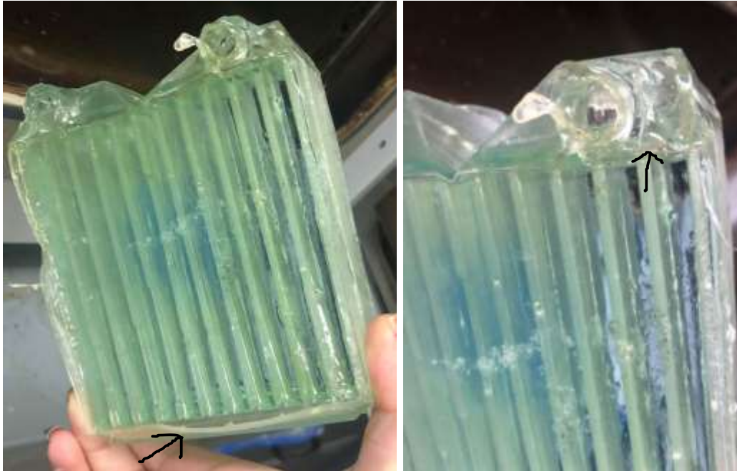
Figure 58: First trial of neat epoxy heat exchanger fabrication- the wax flow channels were entirely removed and there were openings at the bottom of the heat exchanger and by the outlets at the top (marked with black arrows)
