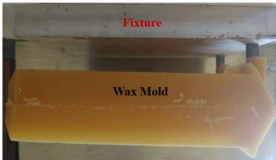
Figure 60: Fixture-wax mold setup
