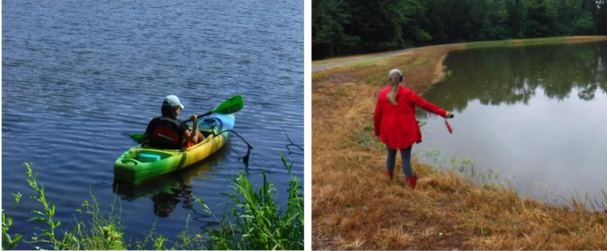
Figure 15: Bathymetric data collection on waterbody in the Southeast Watershed Planning Region of Oklahoma, including the kayak with fish finder mounted on the right side (left). Collection of shoreline global positioning system points used for bathymetric data processing (right).
