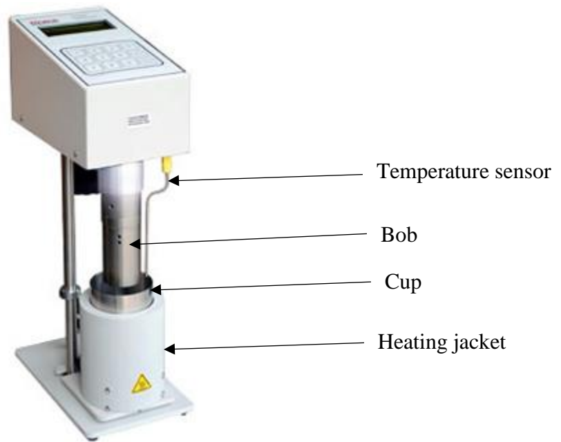
Figure 14- Automatic M3600 viscometer
