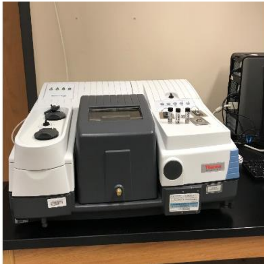
Figure 15- FTIR spectrometer for mineralogy testing
