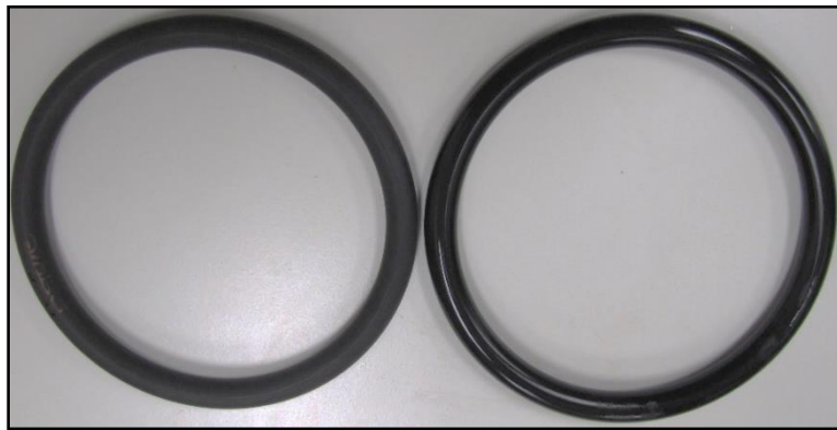
Figure 4.7: EPDM samples before (left) and after (right) surfactant degradation
