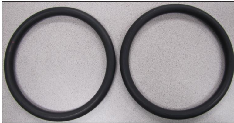
Figure 4.1 : O-ring elastomers to seal the annulus between the inner and outer pipes
