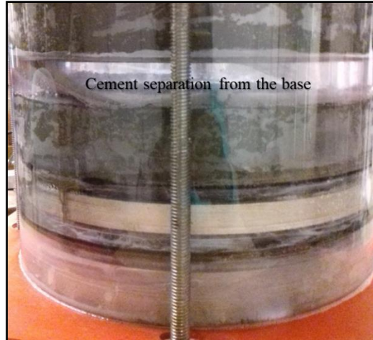
Figure 5.19: Cement separation during the 40-psi pressure test
