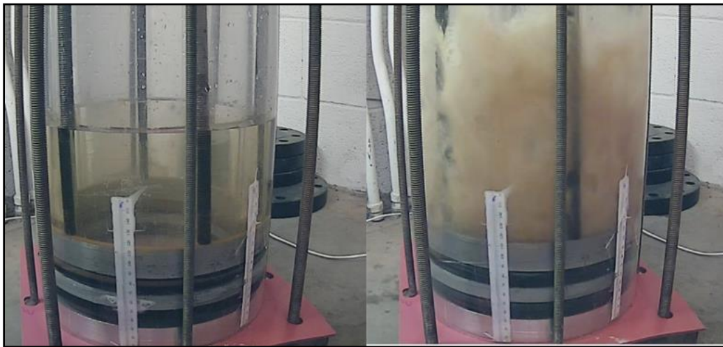
Figure 5.5: NBR pressure cycling test at 180 in-lbf and 120 in-lbf (successful tests)
