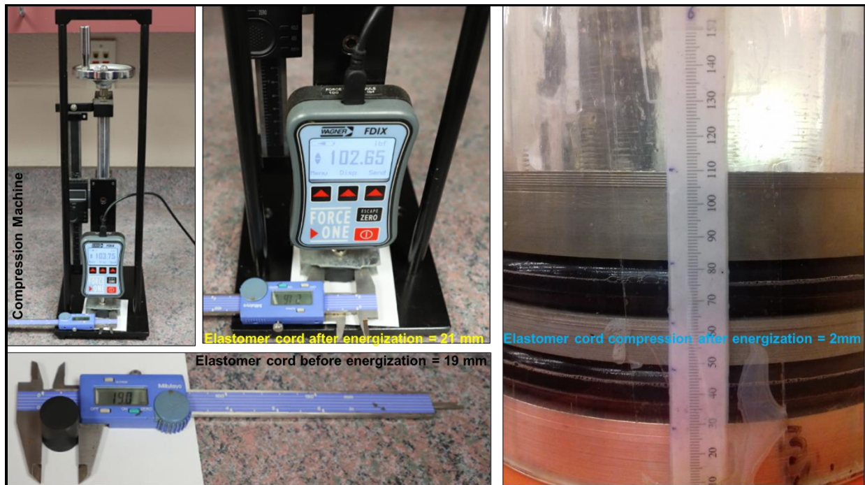
Figure 6.2: Elastomer displacement measurement using compression machine and paper scale
