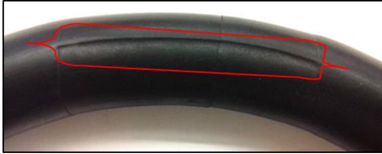
Figure 4.12: Elastomer after creating a seam as an intentional physical defect.
