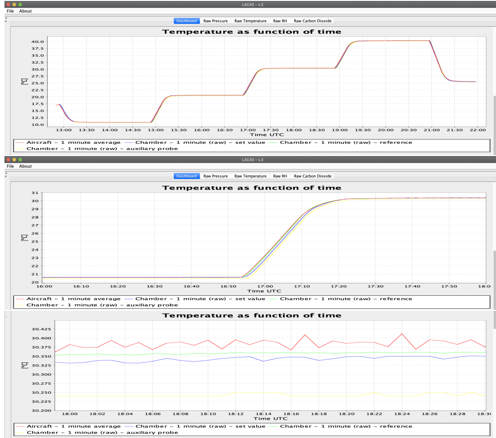
Figure 8.9: LACAS desktop application’s dashboard view of temperature. The top panel shows the set, reference, auxiliary, and LACAS temperature for the entire duration of the experiment. The middle panel shows a detailed view of the 20 °C to 30 °C step transition. The bottom panel shows the detailed view of the dwell part of the 30 °C step. For all plots, the red time series represents the measurements made by LACAS, the green time series represents the chamber reference, the blue time series represents the chamber set values, and the yellow time series represents the temp/RH auxiliary probe.
