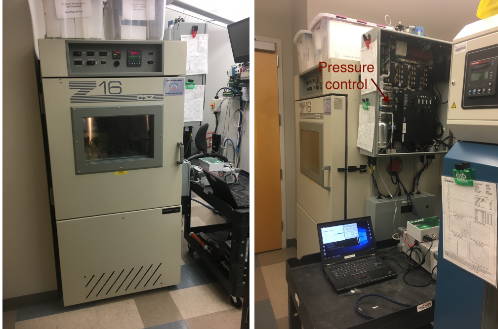
Figure 8.15: The Cincinnati Sub-Zero Z16 environmental simulation chamber (left) with the added gasket-based vacuum and compression system (right).
