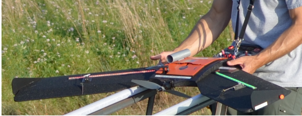
Figure 7.2: The Tuffwing UAVMapper with the LACAS v2 scoop and navigation lights for the flights before sunrise. Photo: Brian Greene.
