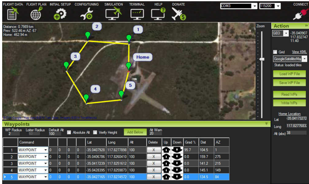
Figure 3.2: Screenshot of the flight programming feature of the Mission Planner software. The top panel shows the mission's waypoints while the bottom panel shows the waypoint action commands.
