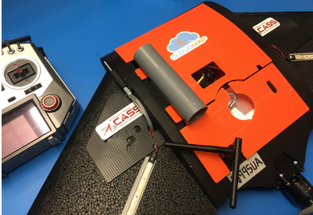
Figure 4.15: The final assembly of the LACAS UAS sensor package v2 on a Tuffwing UAVMapper.
