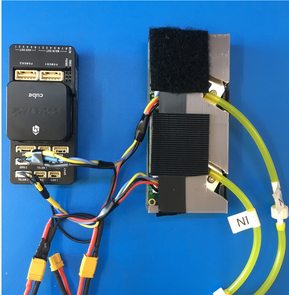
Figure 4.2: Striped-down sensor housing for two K30-FR CO 2 sensor in LACAS v1, with direct wiring to the Pixhawk.
