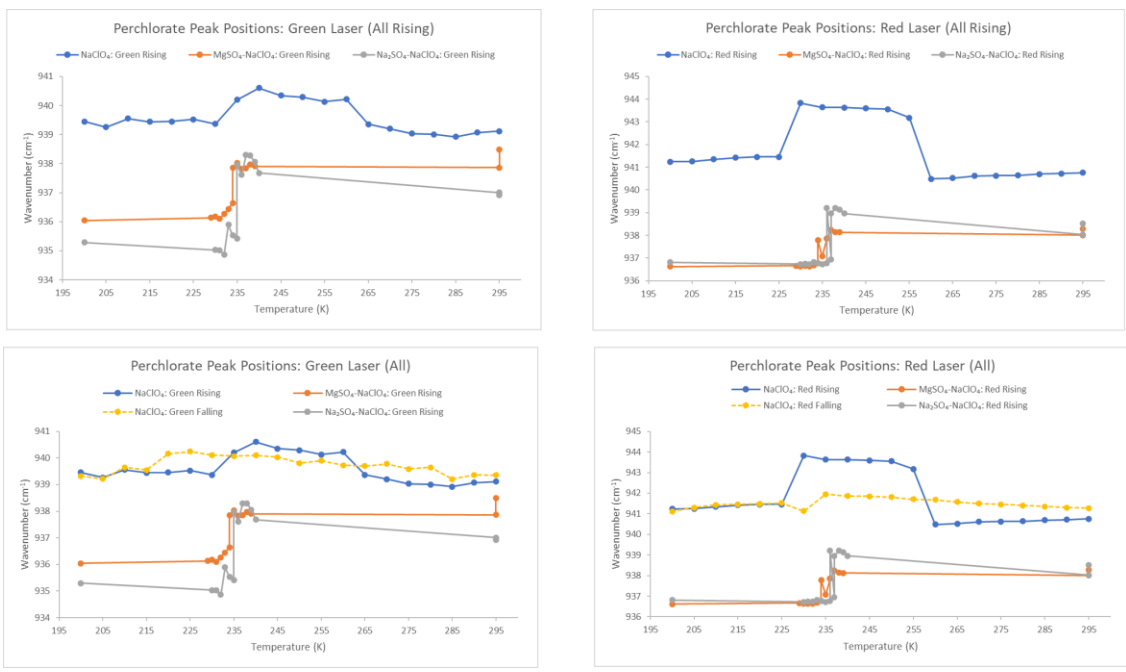
Figure A43: The peak position of the main perchlorate peak for three perchlorate brines using both the 532 nm and 785 nm lasers. Note that plots denoting falling temperatures are denoted by dashed lines, while rising temperatures are denoted by solid lines.
