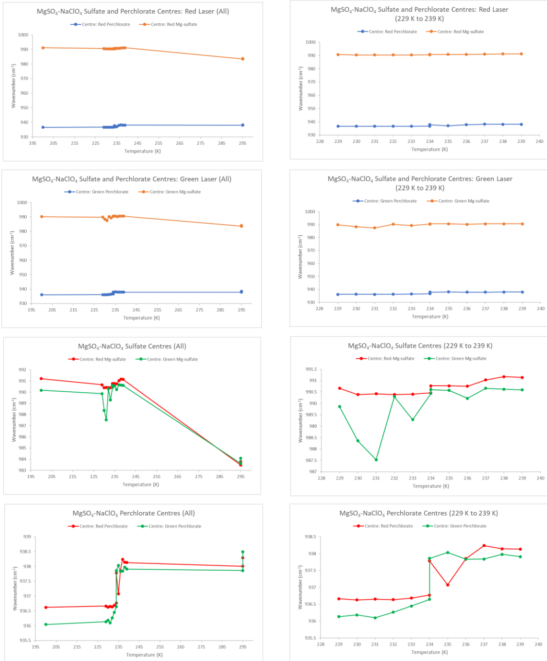
Figure A38: The peak positions of the main sulfate and perchlorate peaks for the MgSO 4 -NaClO 4 brine using both the 532 nm and 785 nm lasers.
