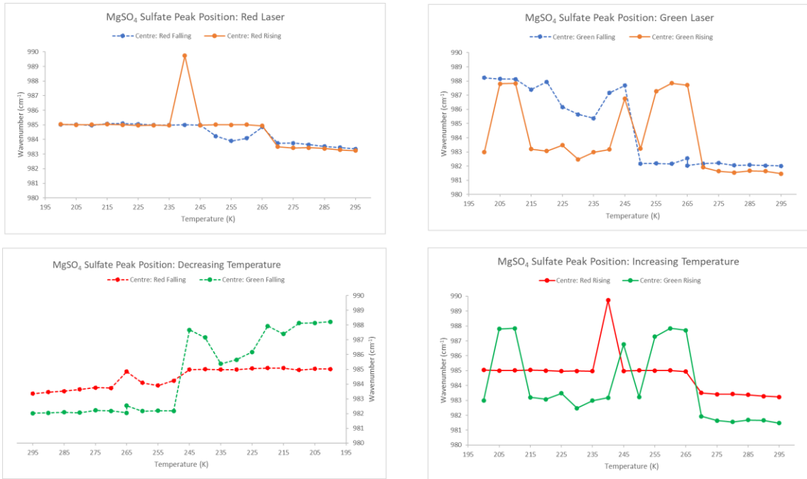
Figure A35: The peak position of the main sulfate peak for the magnesium sulfate brine using both the 532 nm and 785 nm lasers. Note that plots denoting falling temperatures are denoted by dashed lines, while rising temperatures are denoted by solid lines.
