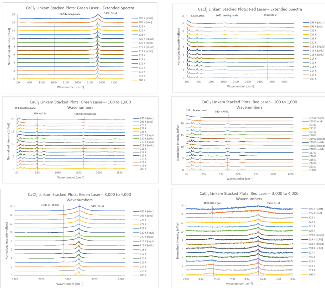
Figure A3: \text{CaCl}_2 stacked plots (green and red lasers), lines and labels included to denote important peaks of ultrapure water (light blue) and \text{CaCl}_2 (purple).
