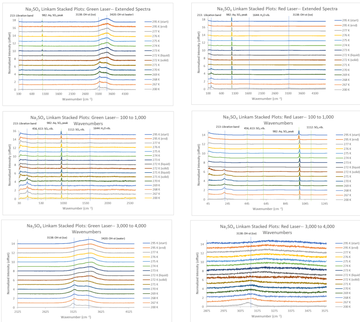
Figure A13: \text{Na}_2\text{SO}_4 stacked plots (green and red lasers), lines and labels included to denote important peaks of ultrapure water (light blue) and \text{Na}_2\text{SO}_4 (light green).
