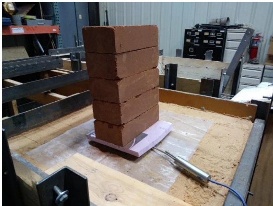
Figure 22. Earth pressure cell calibration
