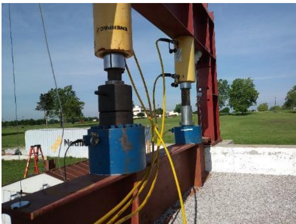
Figure 5. (Left) Load cells during surcharge load testing; (Right) Deconstruction of the models
