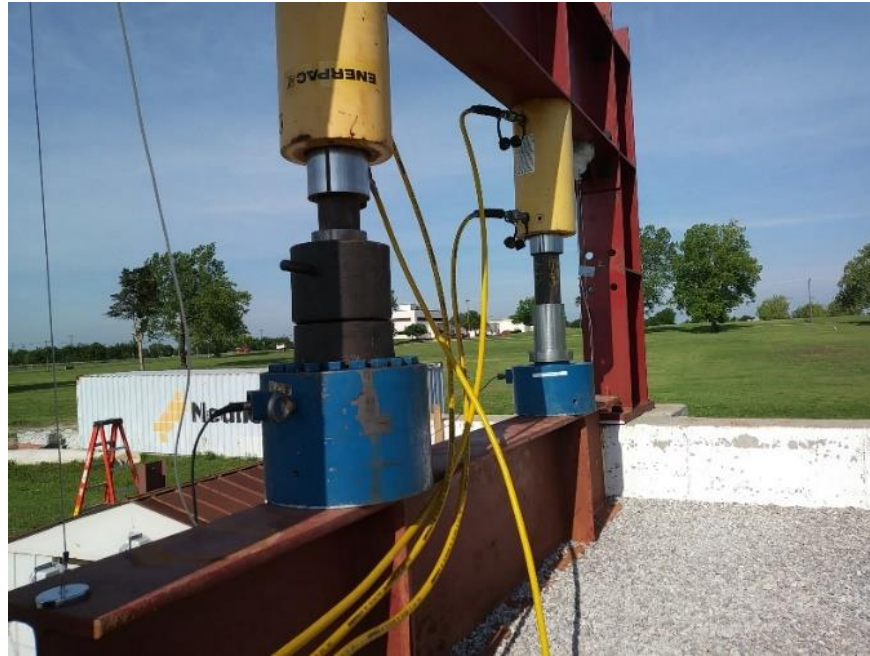
Figure 46. Placement of load cells and their extension blocks before the test
