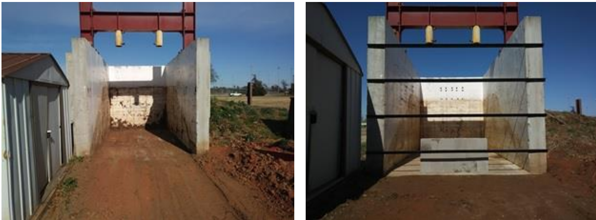
Figure 30. (Left) Front view of OU Fears lab empty full-scale test box; (Right) Front steel frames for WP connections
