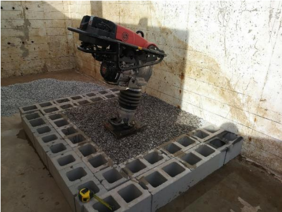
Figure 26. Field evaluation of GRS fill unit weight
