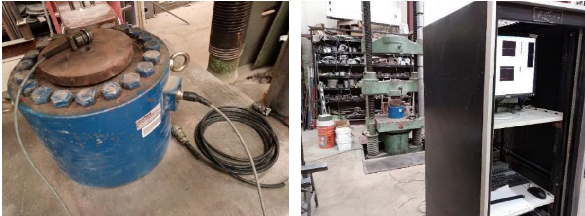
Figure 21. (Left) 400 kip-capacity load cell; (Right) Calibration procedure for the load cell
