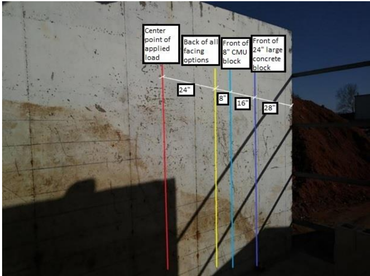
Figure 29. Locations of the loading beam and GRS facing as projected on the sidewalls of the test box
