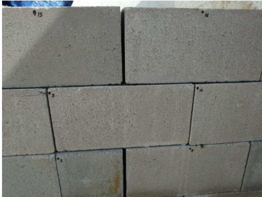
Figure 38. Numbered facing blocks for displacement measurements
