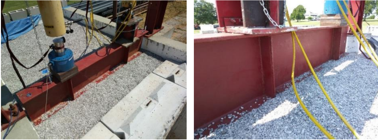
Figure 86. (Left) Top view of the settlement of the loading beam after the test of GRS Abutment Model #2; (Right) Closer view of the loading beam after the test
