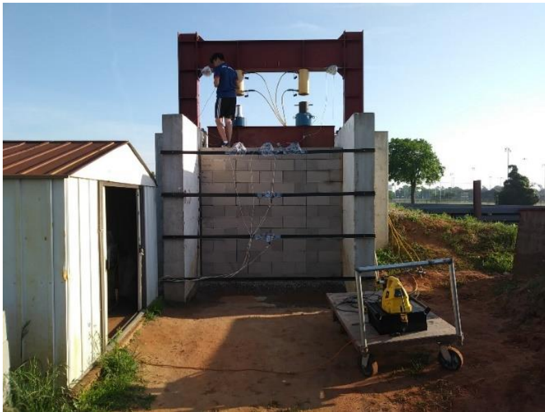
Figure 45. Attachment of the electric-hydraulic pump to the loading assembly
