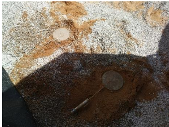
Figure 66. (Left) Instrumented reinforcement at the elevation of 27-inch above the foundation slab; (Right) EPCs located under the first-row of large concrete blocks in GRS Abutment Models #2 and #3
