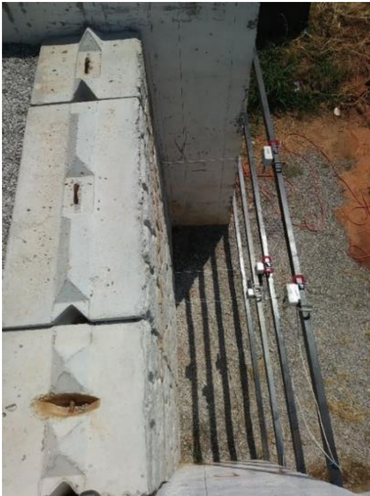
Figure 85. (Top) Front; (Bottom) top views of GRS Abutment Model #2 after the conclusion of its surcharge load testing
