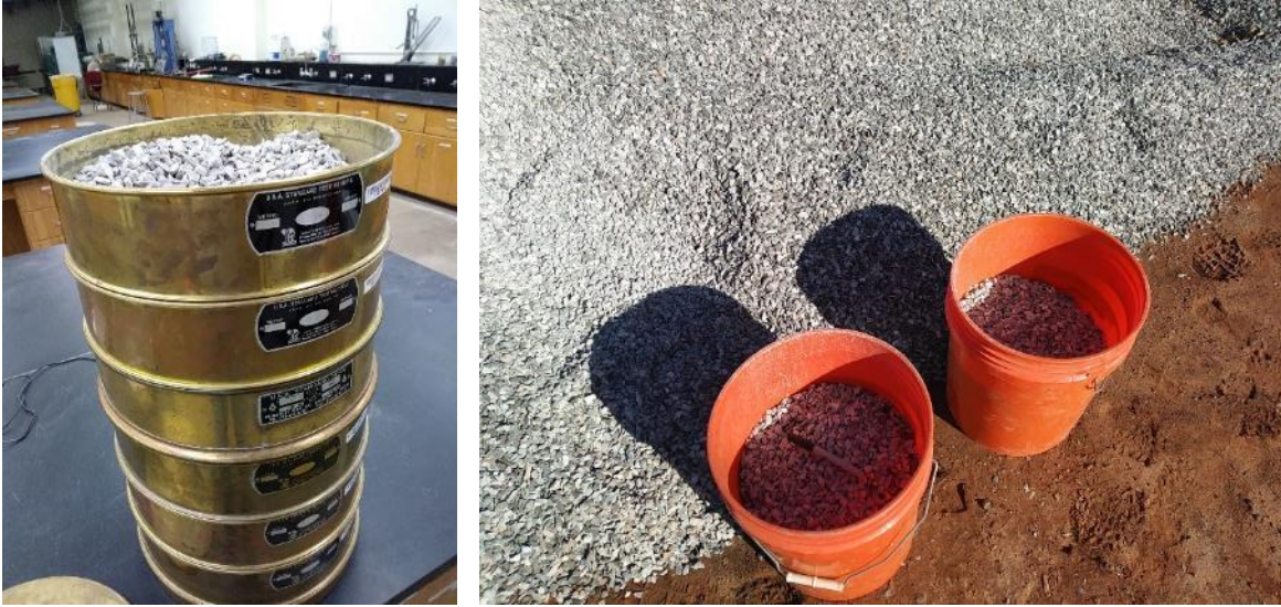
Figure 25. (Left) Sieve analysis of 3/8” #2 Cover aggregate at the lab; (Right) Taking samples of the gravel at site
