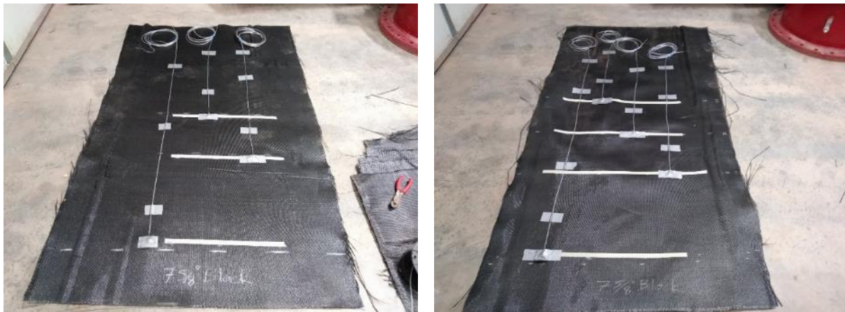
Figure 14. (Left) WP connections at 27-inch level reinforcement layer; (Right) WP connections at 51-inch level reinforcement layer
