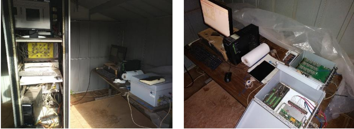
Figure 6. (Left) DAS for WP and LC readings; (Right) Data Loggers for EPC readings
