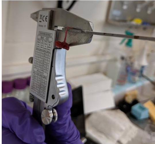
Figure C-4. Measuring the CT thickness with a digital caliper.
