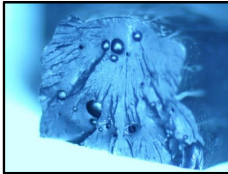
Figure 32: Cross section of non-degassed 10 wt% carbon black, 1 wt% short fiber print
