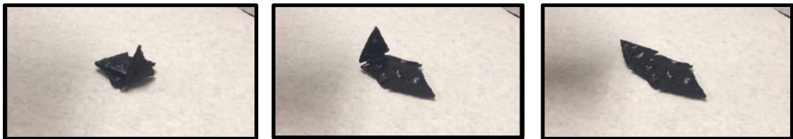
Figure 21: Unfolding process of MWCNT demonstration print
