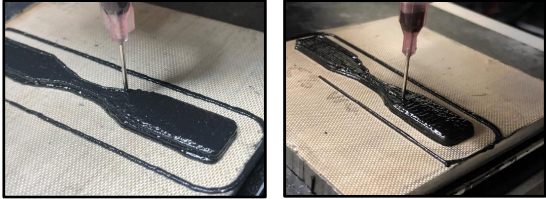
Figure 16: Final layers of dogbone sample being printed
