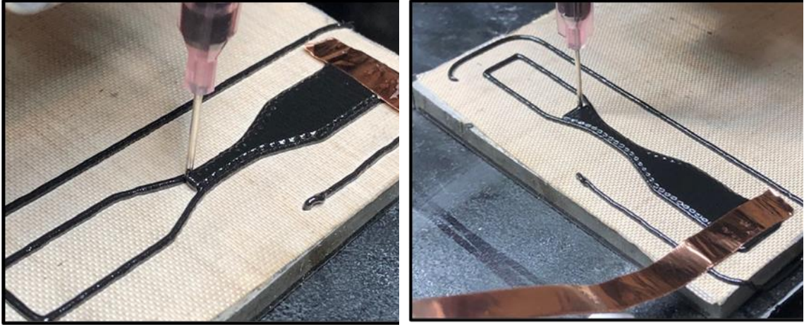
Figure 17: Copper tabs used as electrodes for conductivity testing
