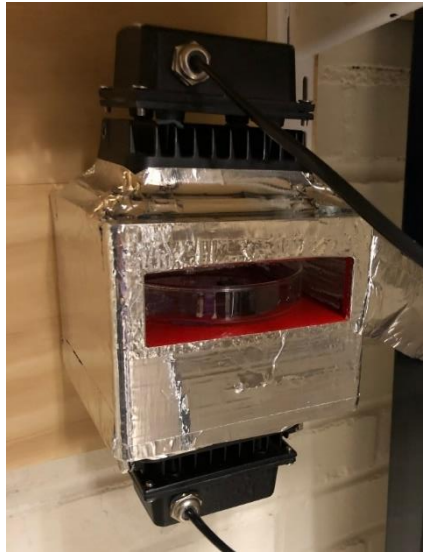
Figure 18: Image of completed UV post-curing chamber
