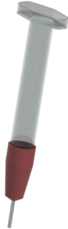
Figure 15: CAD image of syringe with cover attached
