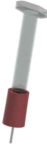
Figure 14: CAD image of syringe with laser shield attached
