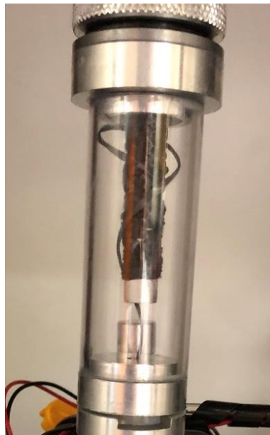
Figure 24: Image of carbon fiber wrapped onto spool and set up on printer
