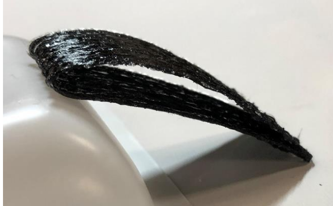
Figure 47: Completed hollow airfoil structure
