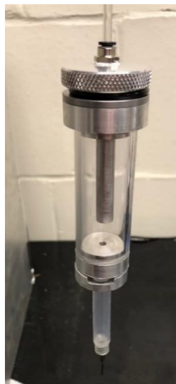
Figure 17: Image of completed fiber chamber with syringe attached
