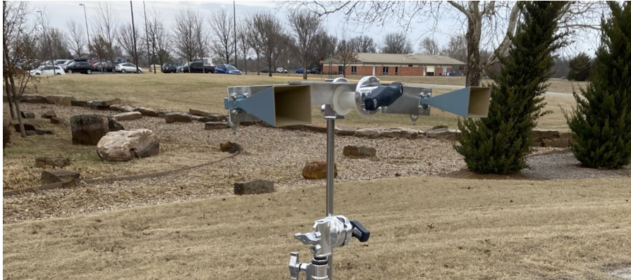
Figure 7.8: The radar set up outside (top) and the mounted quasi-monostatic horn antennae (bottom)
