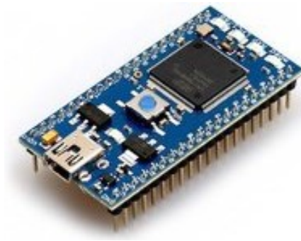
Figure 4.8: The NXP LPC1768 microcontroller
