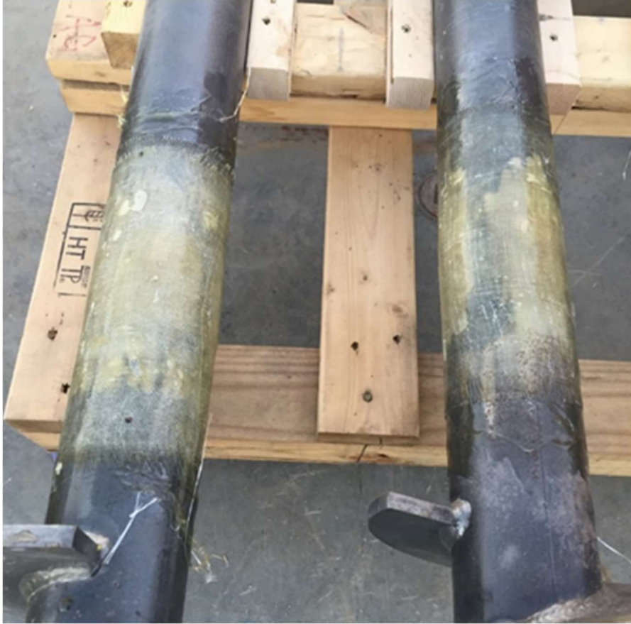
Figure 3.1. Fiber glass fabric and resin wrapped around each strain gage
