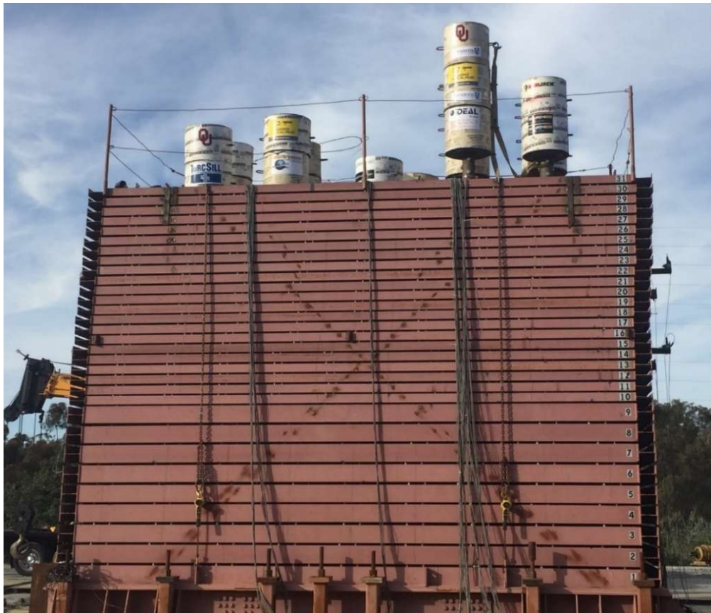
Figure 3.7. Single piles with inertial load on Day 3 of test
