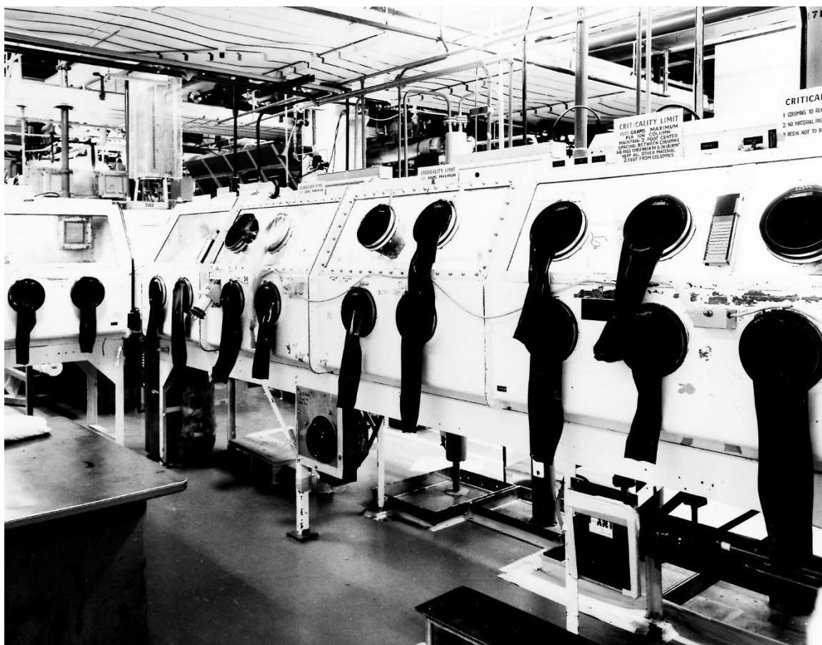
Figure 8: The glove box system in Rocky Flats Plant Building 771. 1960. Image CO-83-N-8. Photograph courtesy of the U.S. Department of Energy.
