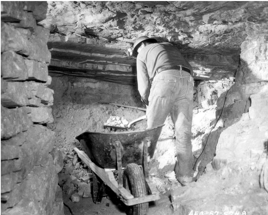
Figure 5: Hand-loading ore in a uranium mine on the Colorado Plateau. c. 1957. Image HD.11D.054. Photograph courtesy of the U.S. Department of Energy.
