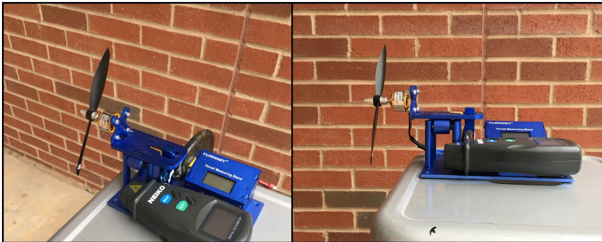
Figure 10: Experimental setup for static, far field thrust measurements
