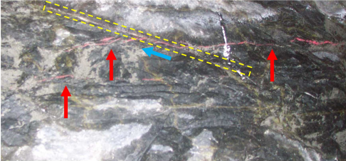
Fig. 4. 6. Mine-back experiment showing HF crossing with a minor offset and a secondary wing-crack propagation parallel to the main HF (Courtesy of Rob Jeffrey, 2001).
