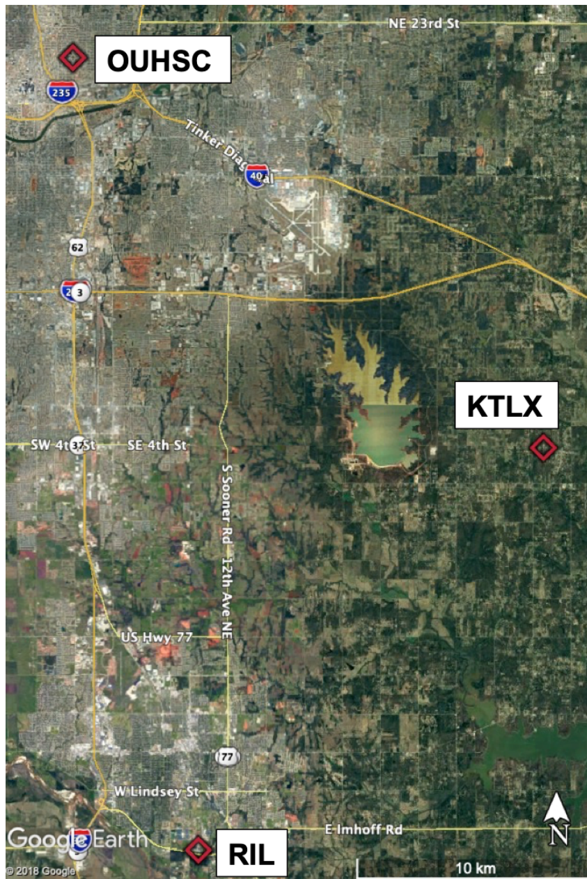
Figure 3.1: This satellite image [44] shows the locations of the two passive receivers at the Radar Innovations Lab (RIL) and University of Oklahoma Health Science center (OUHSC), as well as the location of KTLX, the WSR-88D being utilized as a transmitter of opportunity and also operating as an independent monostatic radar.
