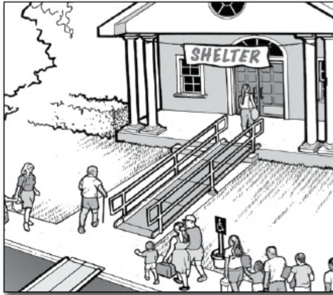
A portable ramp with edge protection and handrails is installed over two steps to provide an accessible route.
