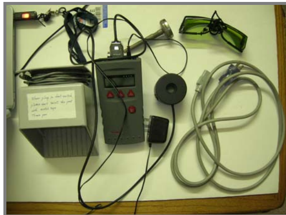
Figure 3.2 Power meter and related devices.
