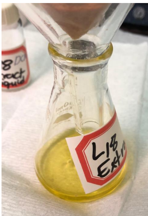
Figure 6.9: Extraction Separation of Lipstick-18 using Dichloromethane
