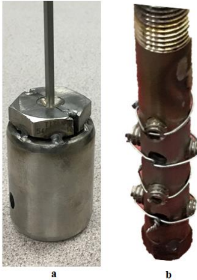
Figure 18. Top spider: a) Initial version b) Final version
