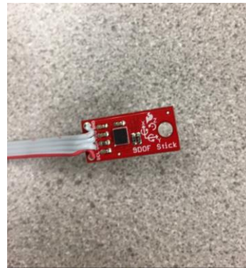
Figure 28. a) DAQ system (Akita et al., 2020) b) Downhole inclination sensor
