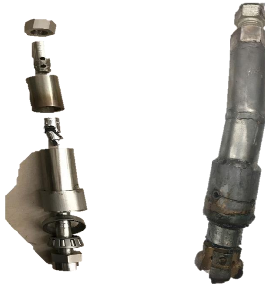
Figure 20. Bent sub and bit assembly: a) interior; and b) exterior
