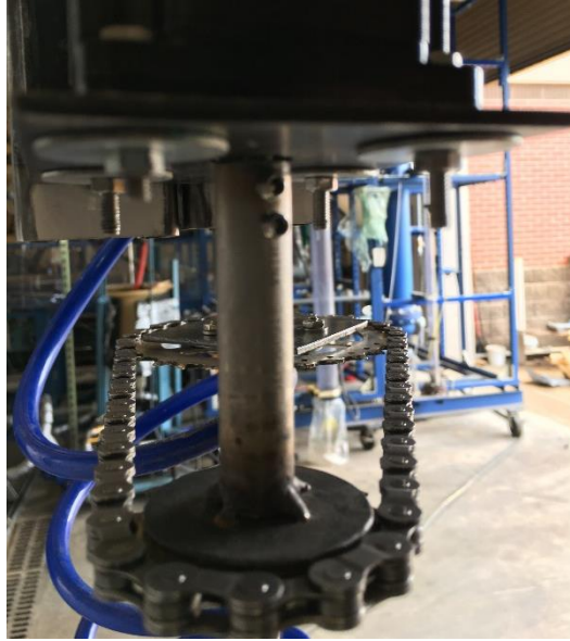
Figure 23. Stepper Motor with Azimuth Control Mechanism (Akita et al., 2020)
