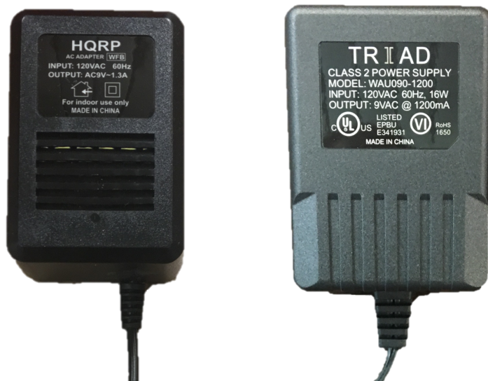
Figure 3.47: Picture of the two 120 VAC-to-9 VAC VTs implemented in the voltage sensors (Triad Magnetics and HQRP).
