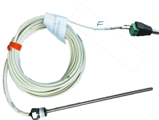
Figure 3.13: In-line, immersion ON-410-PP thermistor modified with DC barrel jack adapters.
