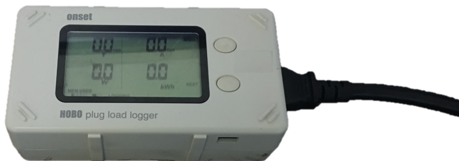
Figure 3.52: Picture of the HOBO UX120-018 Plug-Load Data Logger used with the in-line energy meter.
