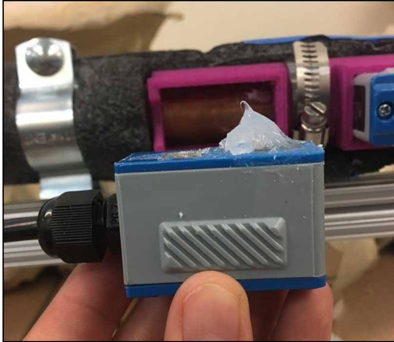
Figure B.1: Acoustic couplant added to bottom of transducer.
