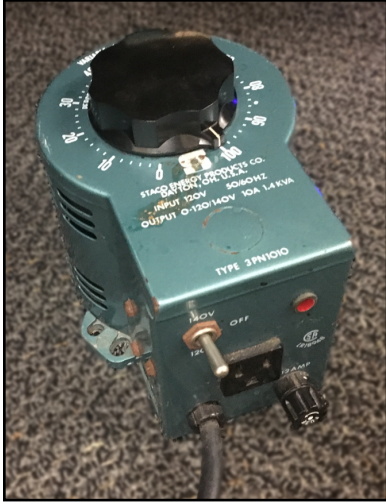
Figure 3.55: Picture of the VARIAC 120/140 VAC power transformer used. Figure 3.56: Picture of a spliced extension cord modified for a CT to measure current passing through one wire of the cable.
