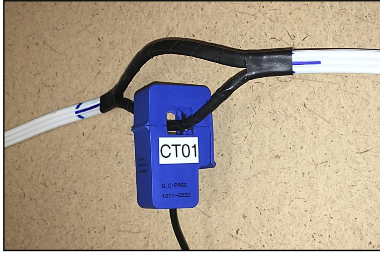
Figure 3.55: Picture of the VARIAC 120/140 VAC power transformer used. Figure 3.56: Picture of a spliced extension cord modified for a CT to measure current passing through one wire of the cable.
