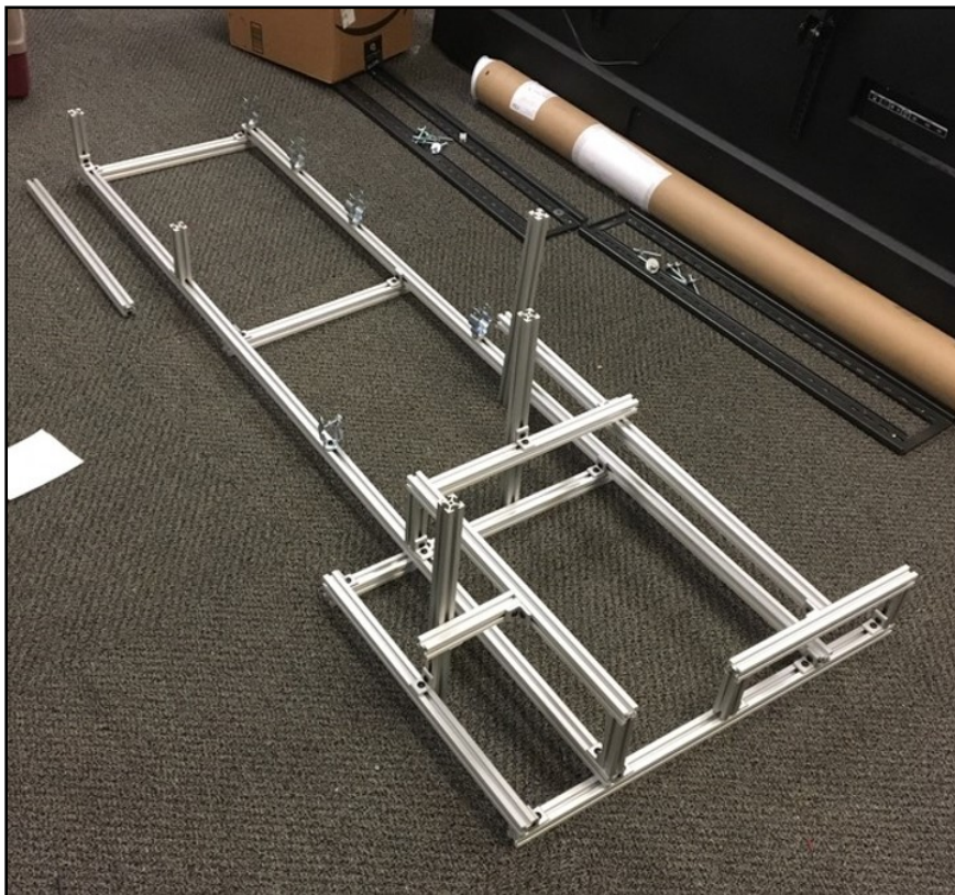
Figure 2.19: 80/20 aluminum extruded frame being assembled.
