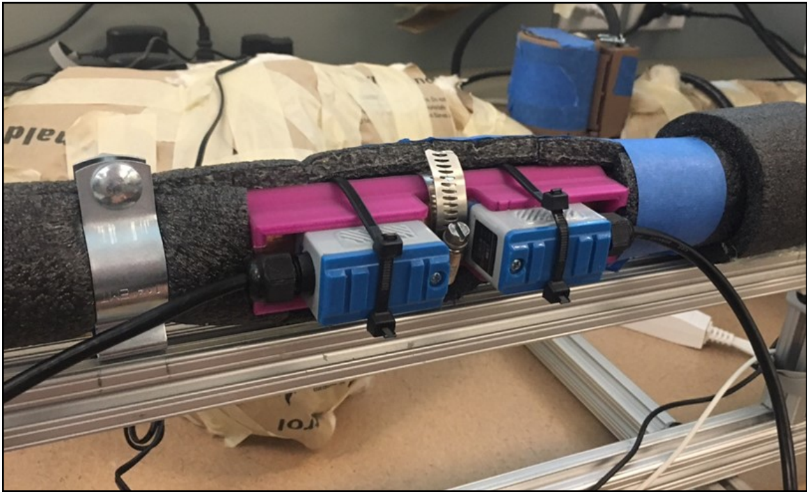
Figure B.4: Mounted transducers, using custom 3D-printed alignment tool (isometric view).
