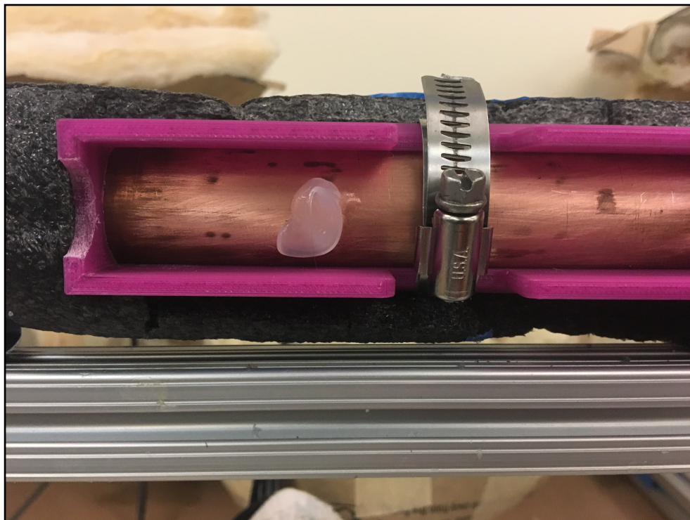
Figure B.2: Acoustic couplant added on the polished pipe.
