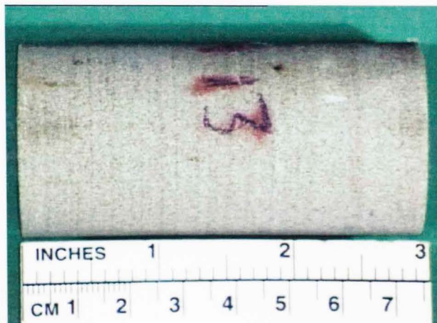
Figure AIV.6 Photograph of sample H13 showing ductile failure. ( \sigma_c = 3.45 MPa; \sigma_{fail} = 95.9 MPa Porosity = 19.1%; k = 150 mD; \beta \approx 90^\circ ).
