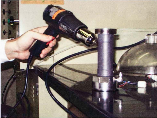
Figure 3.9 Preparation of the sample. Heating the polyolefin tube on the sample to provide an impermeable barrier to confining pressure.
