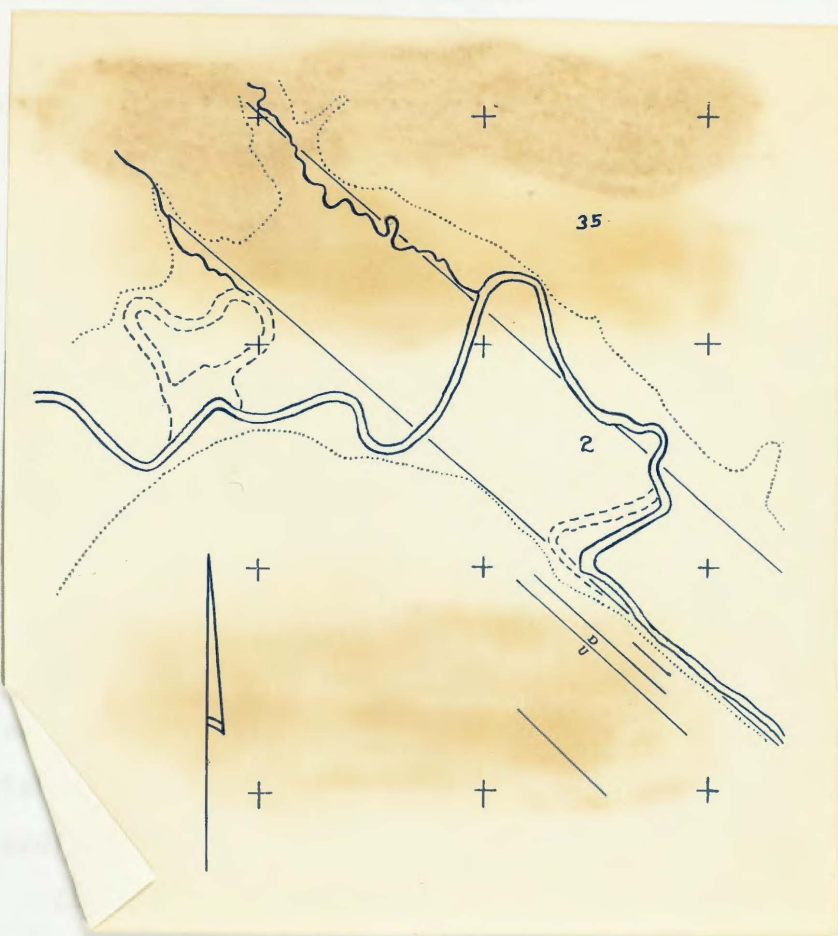
Figure 17. A graben inferred from aberrations in the behavior of the North Canadian River. Sec. 2 is in T. 11 N., R. 8 E. Among the faults southwest of, and parallel to, the supposed graben are several with sufficient displacement to be measured by reconnaissance methods. The presence of this fault system makes precise correlation of the Dewey and Belle City formations difficult.
