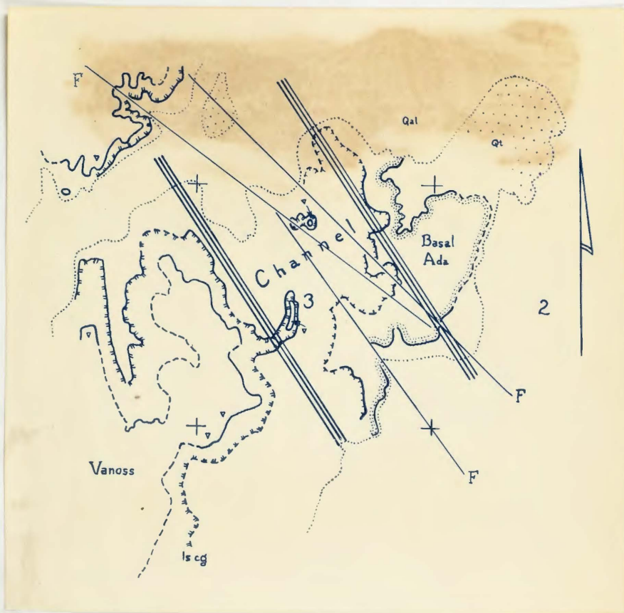
Figure 24. A channel at the base of the Vanoss formation, in sec. 3, T. 6 N., R. 6 E. The basal Ada sandstone is outlined by a double row of dots; two units within the middle Ada limestone conglomerate zone are indicated by two distinct hachure patterns; and arkose outcrops in the basal Vanoss member are shown by small triangles. Section-corner crosses provide a scale. The channel is at least 1,800 feet wide, and about 30 feet deep; the current probably flowed from the southeast to the northwest.
