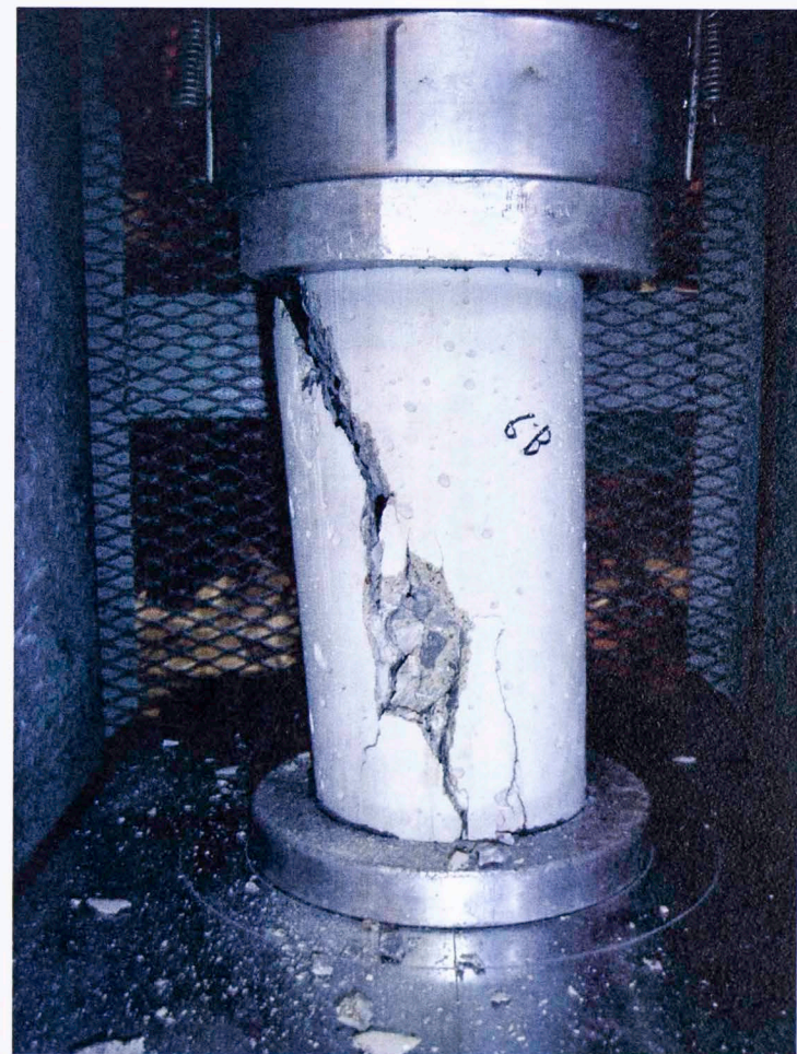
Figure 34 - Cylinder Failure after 28 Days
