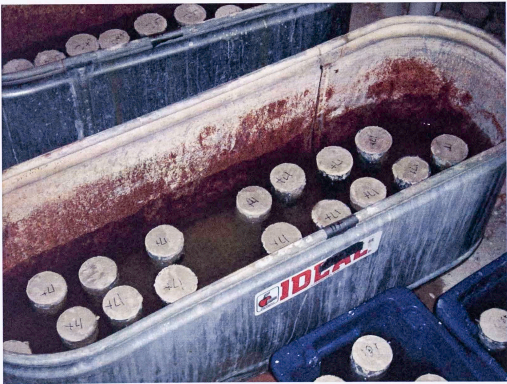
Figure 13 - Small Stock Tanks for Sixty Degree Curing
