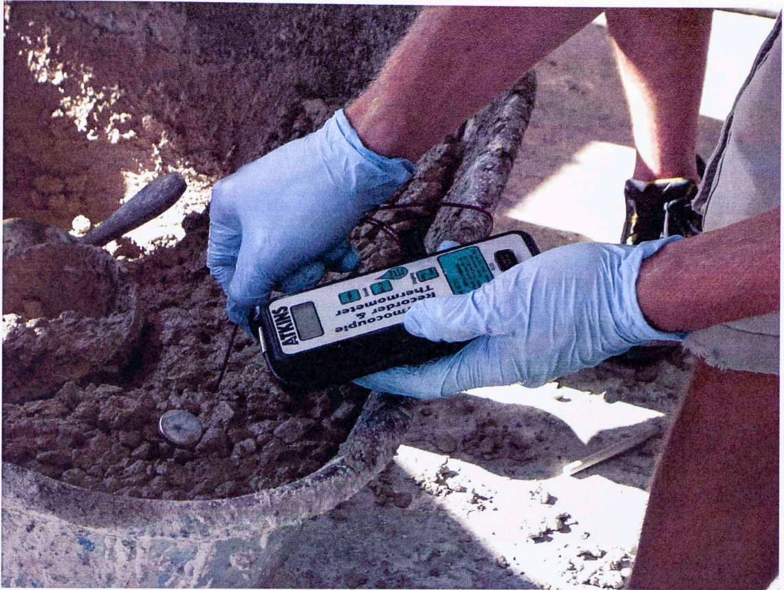
Figure 25 - Taking Temperature Using a Thermocouple and Analog Thermometer
