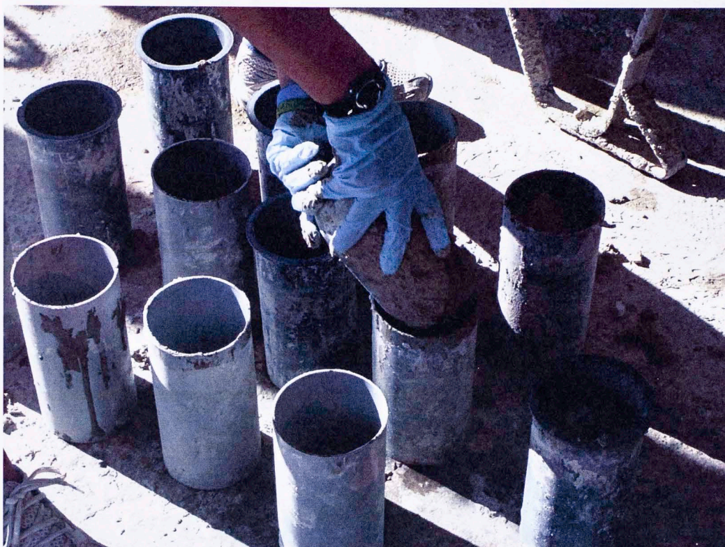
Figure 21 - Filling Cylinder Molds
