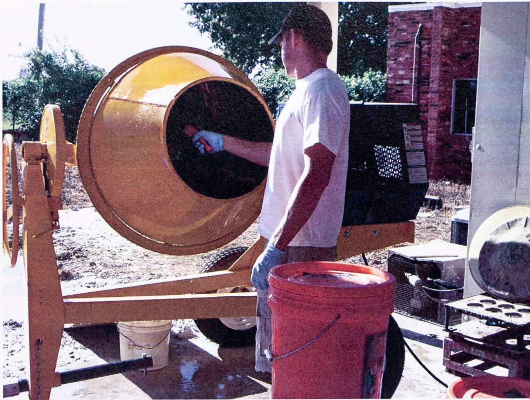
Figure 9 - Measuring Temperature of Mixer Using Infrared Thermometer
