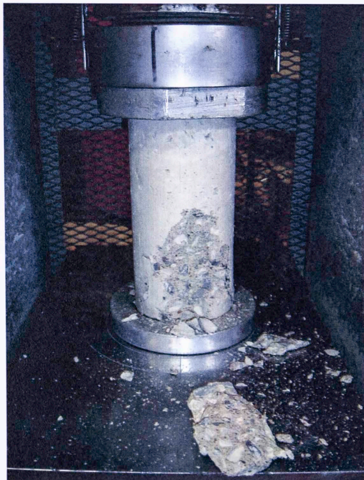
Figure 33 - Cylinder Failure after 6 Hours
