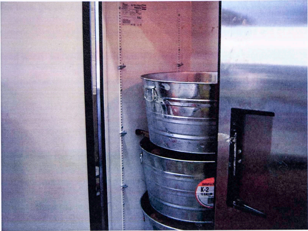
Figure 12 - Water Basins in Freezer for Forty Degree Curing
