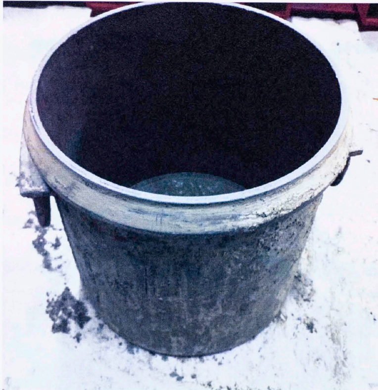
Figure 29 - Air Content Pot Used for Unit Weight
