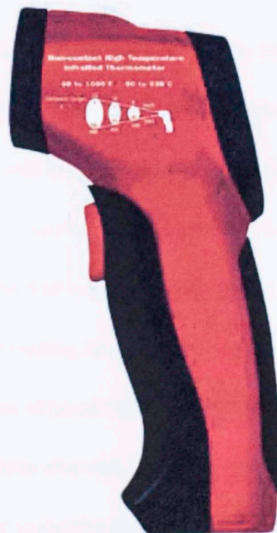
Figure 8 - Infrared Digital Thermometer
