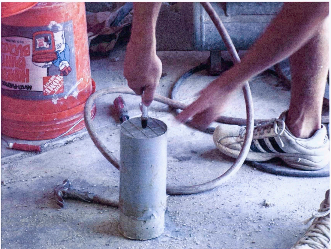
Figure 30 - Removing a Sample from Cylinder Mold Using a Compressed Air
